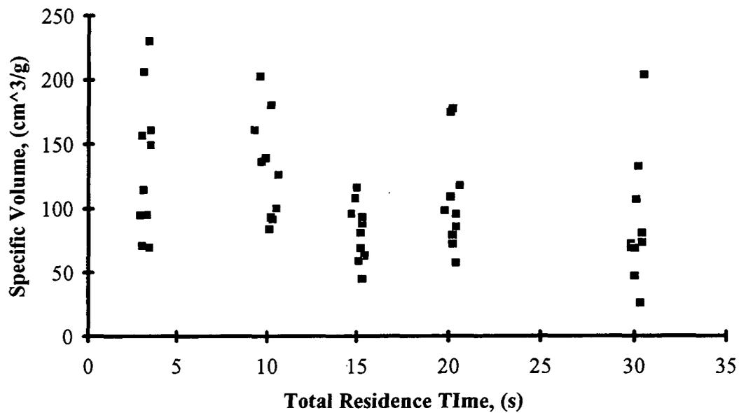
Figure 10: Specific Volume of Kraft Black Liquor as a Function of Total Residence Time in 5%CO/95%N<sub>2</sub> at 900°C and 0.61 m/s
