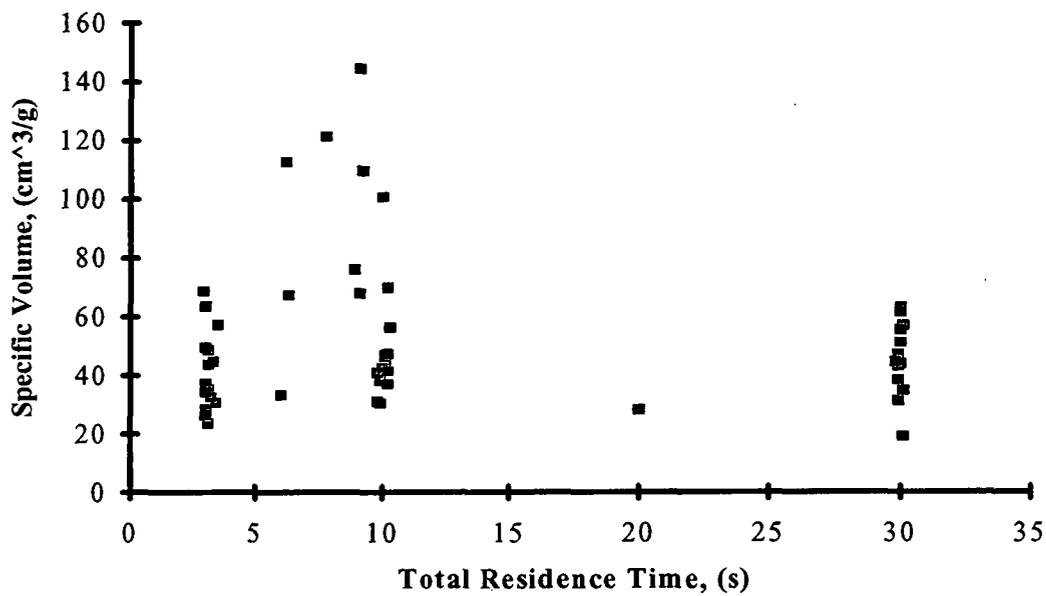
Figure 9: Specific Volume of Kraft Black Liquor as a Function of Total Residence Time in 5%CO/95%N<sub>2</sub> at 750°C and 0.61 m/s
