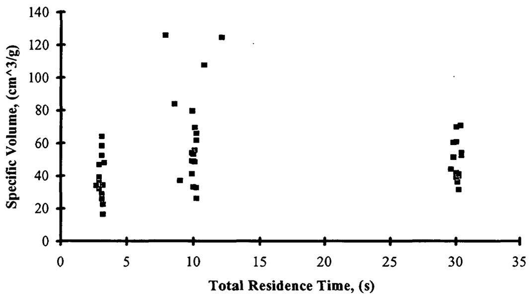
**Figure 11: Specific Volume of Kraft Black Liquor Char as a Function of Total Residence Time in 5%CO/95%N<sub>2</sub> at 750°C and 1.83 m/s.**
