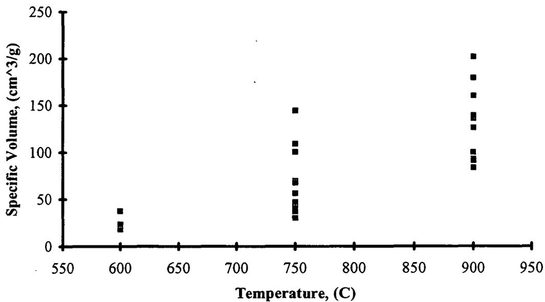
**Figure 5: Specific Volume of Kraft Black Liquor Char as a Function of Temperature in 5%CO/95%N<sub>2</sub> at Exposure Time of 10 Seconds and Gas Velocity of 0.61 m/s.**
