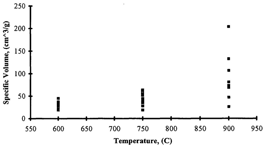
**Figure 6: Specific Volume of Kraft Black Liquor Char as a Function of Temperature in 5%CO/95%N<sub>2</sub> at Exposure Time of 30 Seconds and Gas Velocity of 0.61 m/s.**
