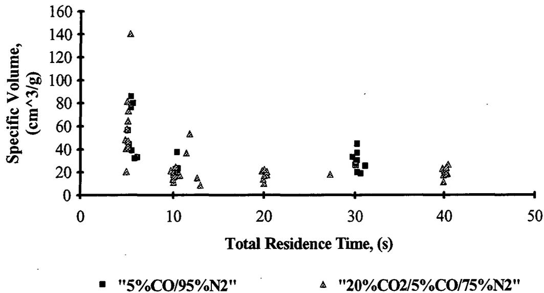
Figure 7: Specific Volume of Kraft Black Liquor as a Function of Total Residence Time at Gas Conditions of 600°C and 0.61 m/s.
