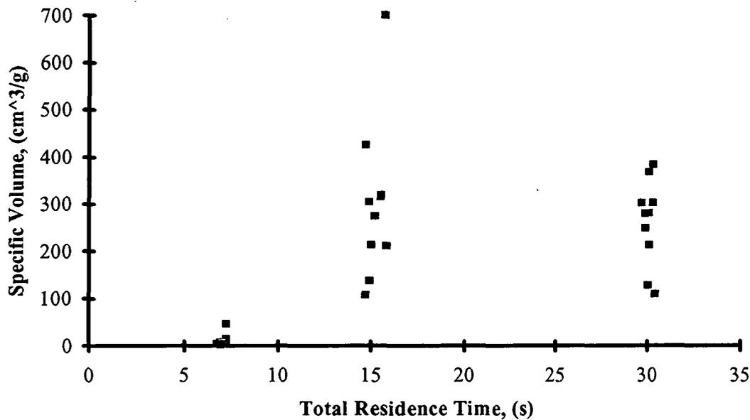
Figure 8: Specific Volume of Kraft Black Liquor as a Function of Total Residence Time in 5%O<sub>2</sub>/95%N<sub>2</sub> at 500°C and 0.61 m/s
