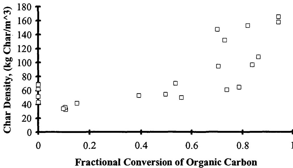
**Figure 4: Bulk Density of Char as a Function of Fractional Conversion of Organic Carbon.**
