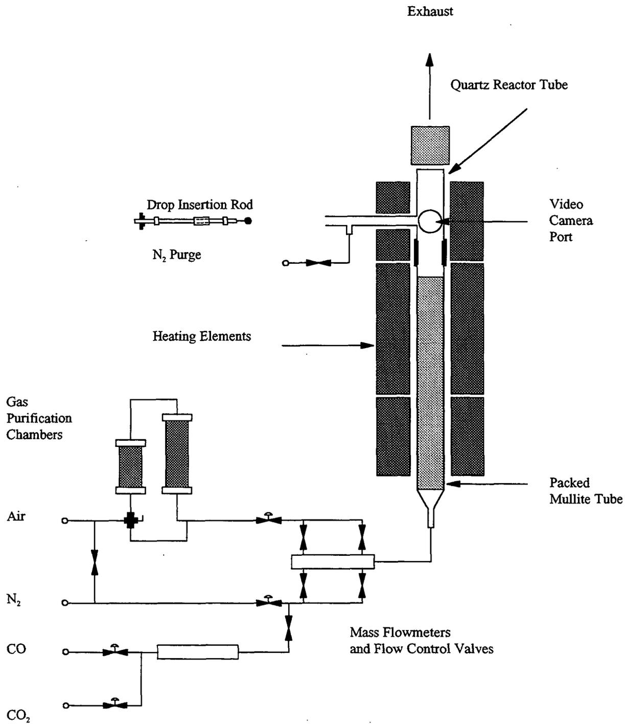
Figure 2: Schematic for Single Particle Reactor Used for Swelling Experiments[15].
