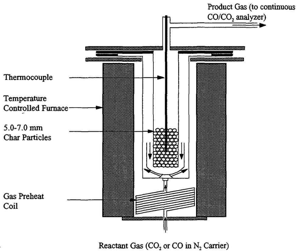
Figure 1: Schematic for Fixed Bed Reactor Used for CO<sub>2</sub> Gasification of Black Liquor Char[13].
