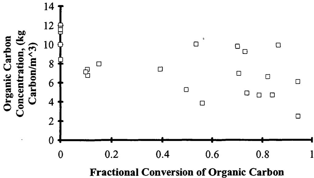
**Figure 3: Concentration of Organic Carbon as a Function of Fractional Conversion of Organic Carbon.**
