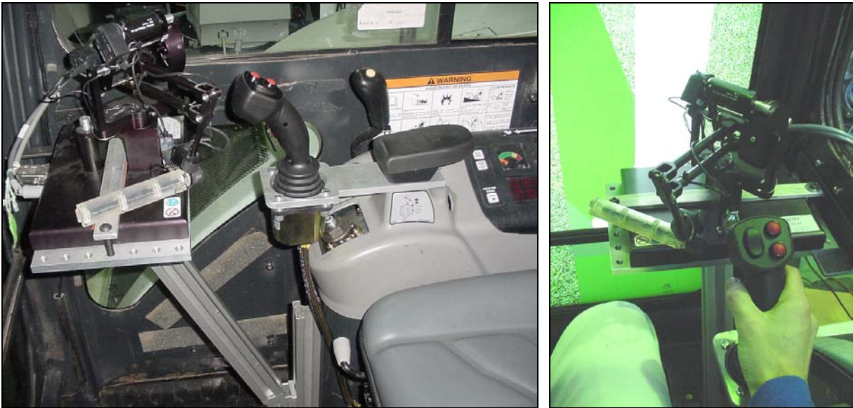
Fig. 3: Phantom and right hand joystick mounted and in use in the operator workstation
