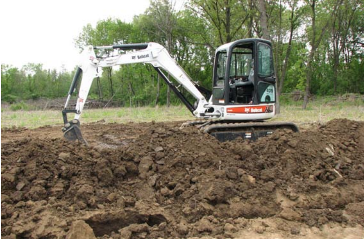
Fig. 1: The pump-controlled Bobcat 435 excavator modelled in simulation
