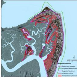
Figure 5.4- Hard Structural Protection Alignment for Wilmington Island, Potential
