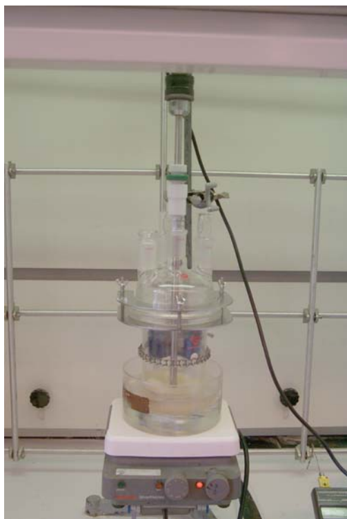
Figure 3.7: Mixed matrix dope mixing setup
