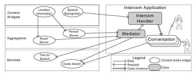
Figure 1 Intercom Application Software Design.
