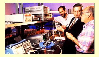
Rob Pauley (left), Dr. Gene Greneker (center) and Bruce Warren (right) examine a radar detector. They are investigating how to send encoded signals that detectors would decode and convert into traffic hazard warnings for drivers.
