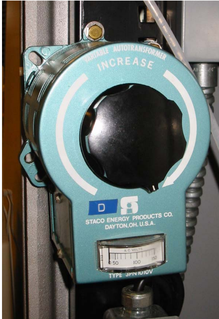
Figure 3.49 Staco Energy Products Model 3PN1010V Variable Autotransformer Input 120 Vac, Output 0-140 Vac, Rated for 10 Amp / 1.4 KVA.
