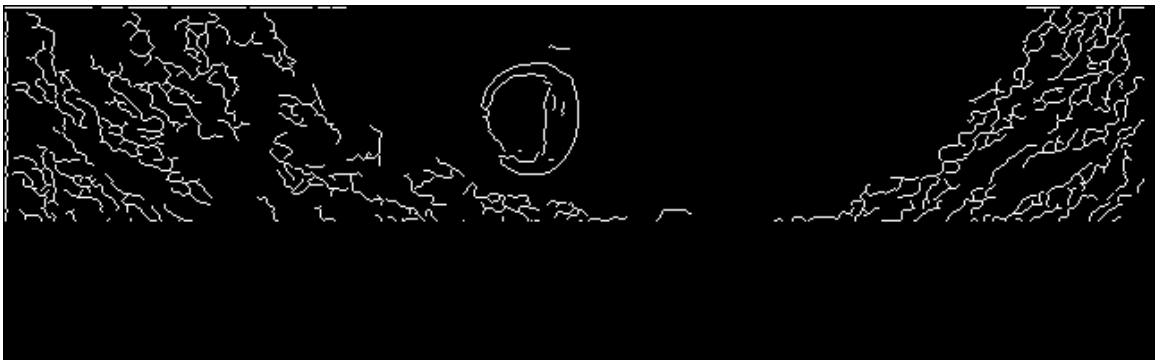
Figure 3.72 Example of Incomplete Droplet with Threshold set to 0.15 (15FEB#8-8).
