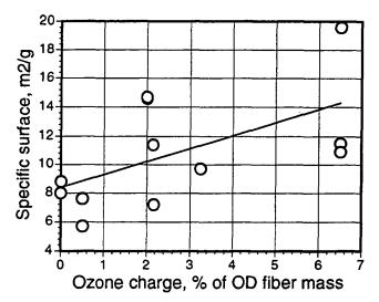
Figure 3. Relationship between ozone charge and sheet specific surface for bulk ozonated pulp.
