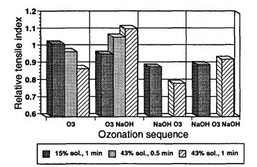
Figure 5. Effect of ozonation sequence on ozonated sheet tensile index.
