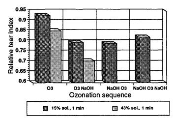
Figure 6. Effect of ozonation sequence on ozonated sheet tear index.
