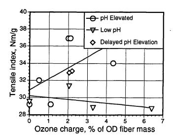
Figure 2. Tensile versus ozone charge for three different pH treatments.
