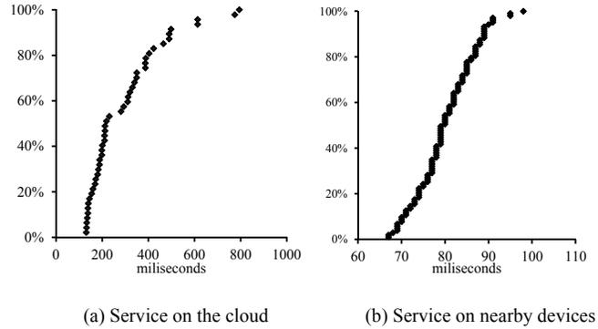
Figure 5. Cumulative distribution functions of network delay when the service runs on the cloud ( $EC2$ ) and on a nearby device ( $N1, N2$ ), respectively.
