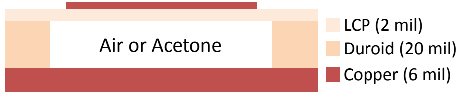
Fig. 6.4 2D cross sectional view of the stack-up.
