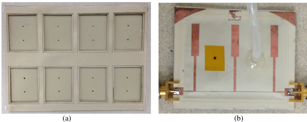
Fig. 5.7 a) Layers stack-up before lamination b) Fabricated tunable filter.
