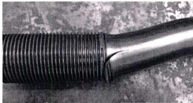
Figure 5. Point of fracture of the compression only specimen tested dynamically at a loading rate of 1.3 mm/sec (0.05 inch/sec)
