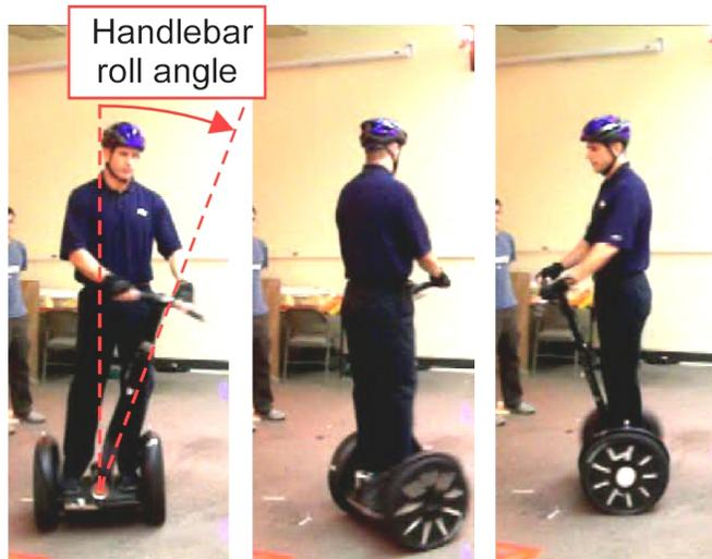
**Figure 3.34:** Spinning Test on a Segway i2.
