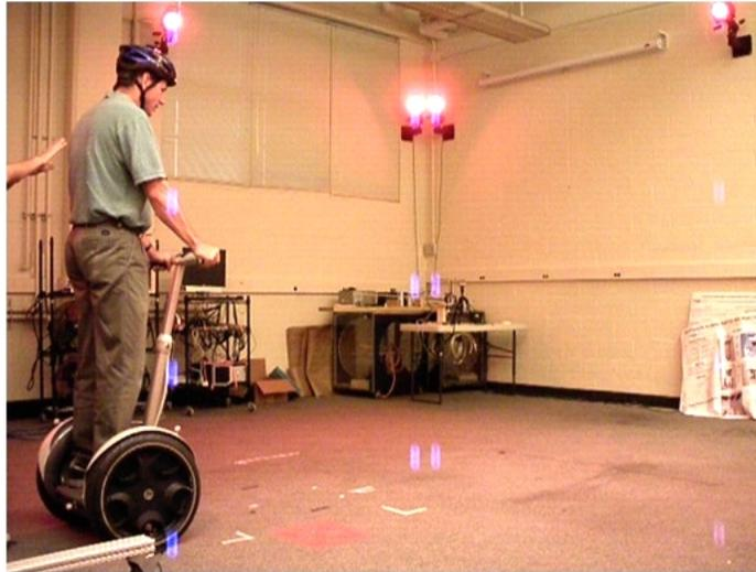
**Figure 3.6:** Manual pulse force applied on a loaded Segway i167.
