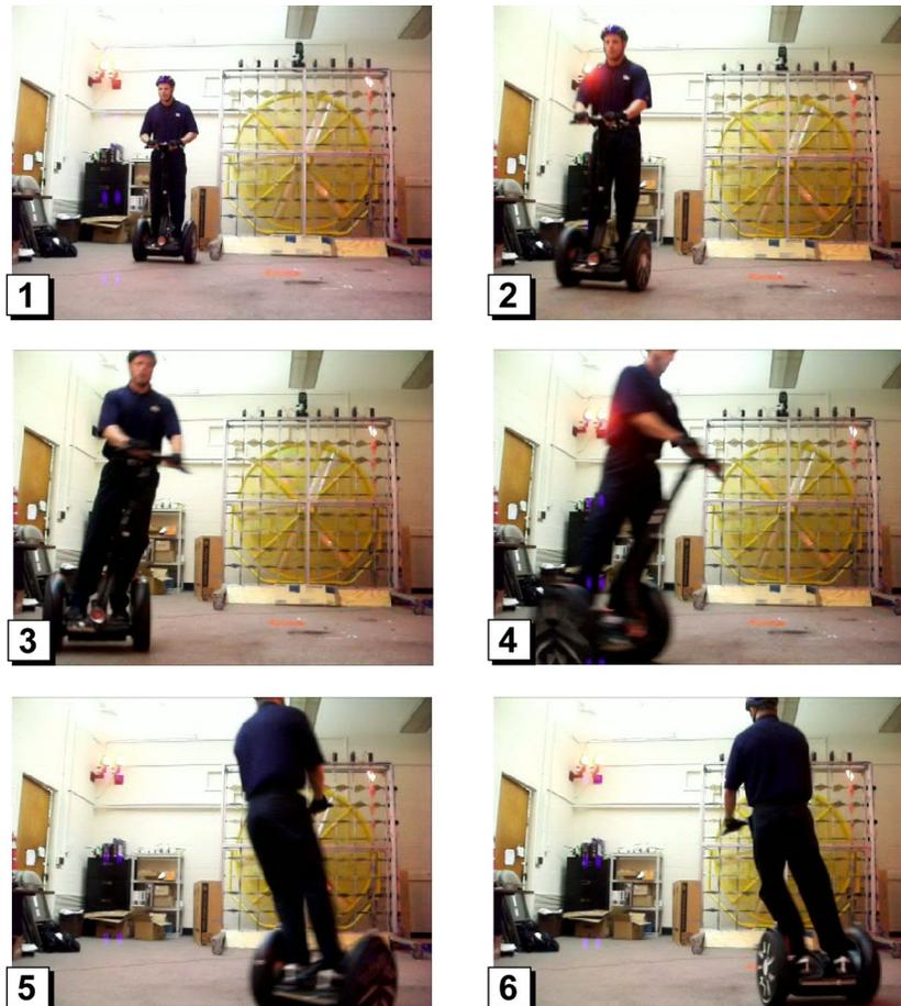
Figure 3.9: Turning test on a Segway i2.
