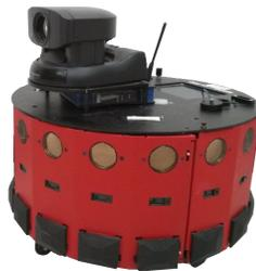
Figure 27: Shown is a picture of the IRobot Magellan-pro.
