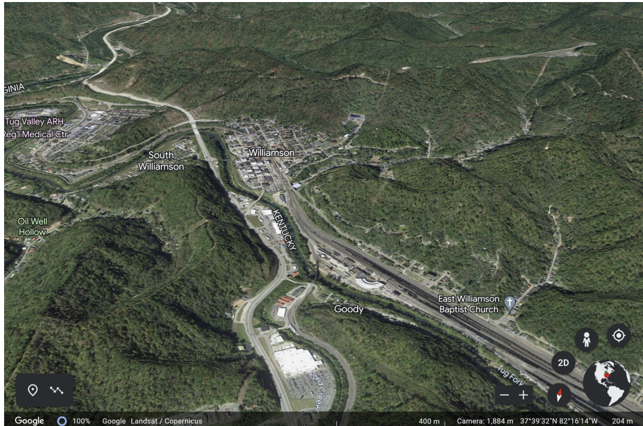
Figure 7. Google Earth 3D axis view of Williamson, WV to highlight the extreme topography changes that contribute to fast flooding of lower valley towns (Sourced from Google Earth 2023).
