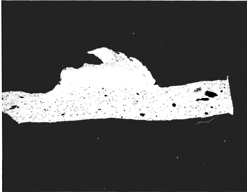
Figure 14. ATR Dispersion Sag Tested by 1710^{\circ} F (7x).
