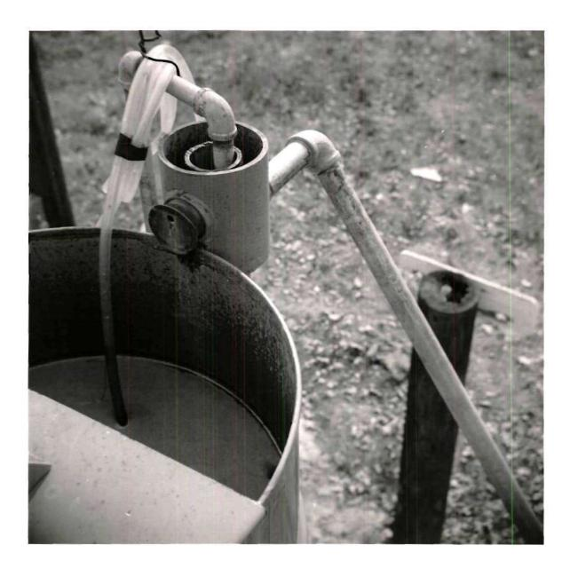
Figure 7. Picture of the Constant Head Orifice
