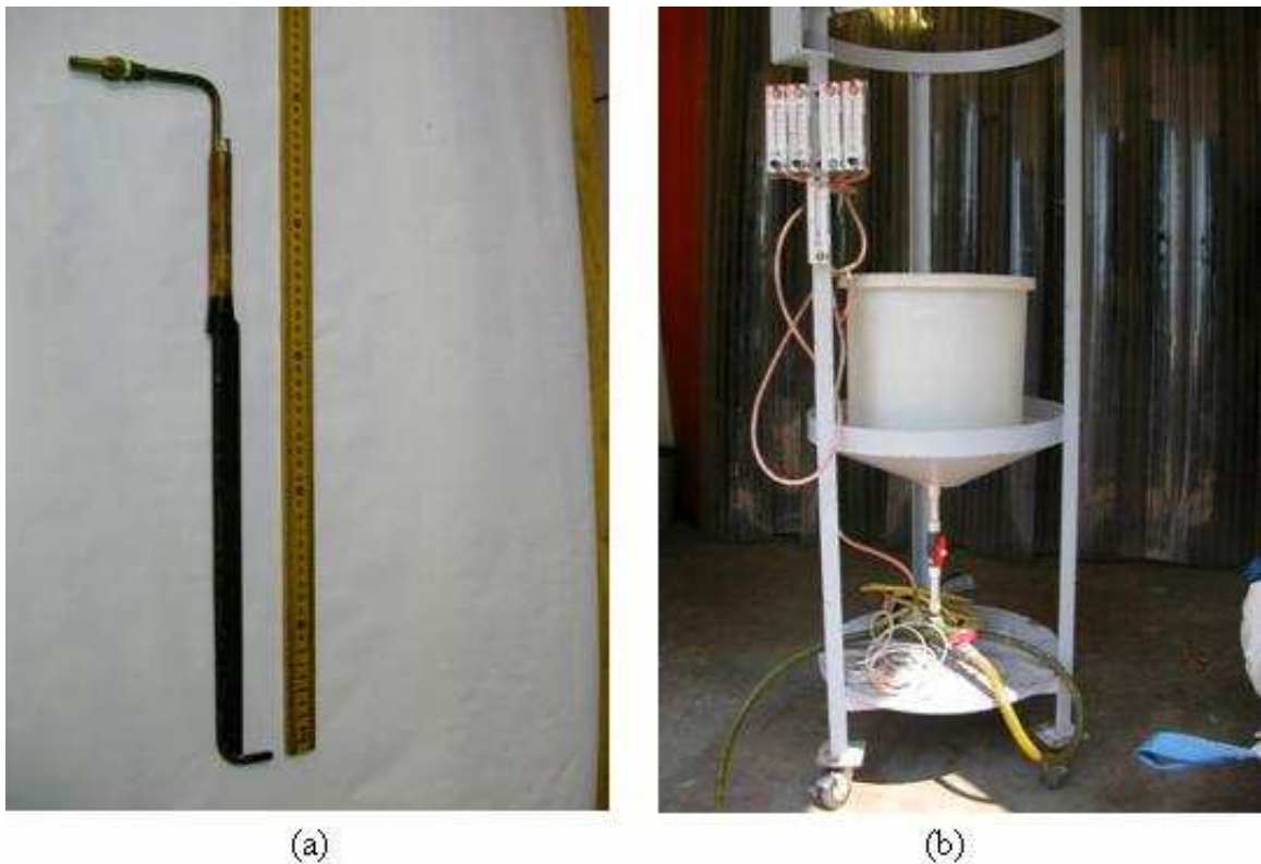
Figure 4.10 Tracer delivery system: (a) the brass effluent nozzle and (b) pump stand with 30 liter conical bottom tank and rotameter
