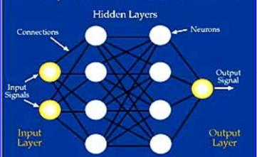
Neural neworks are typically organized in layers. Layers are made up of a number of interconnected "nodes" that contain an "activation function." Patterns are presented to the network via the "input layer," which communicates to one or more "hidden layers" where the actual processing is done via a system of weighted "connections." The hidden layers then link to an "output layer" where the answer is output as shown in this graphic. (Click on the image to see larger 38k version).
