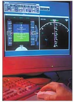
Cockpit Display of Traffic Information technology would provide an enhanced cockpit display that allows pilots to see other aircraft around them and the distances between them. (300-dpi JPEG version - 585k)
