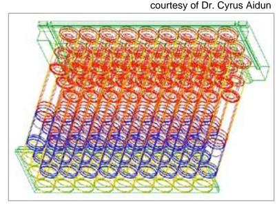
A new technology is strengthening paper fiber, while lowering the energy costs of manufacturing it. A device that is retrofitted into an existing paper machine's headbox (shown here) disperses wood fibers uniformly in all directions, strengthening the paper. <u>(300-dpi JPEG version -546k)</u>
