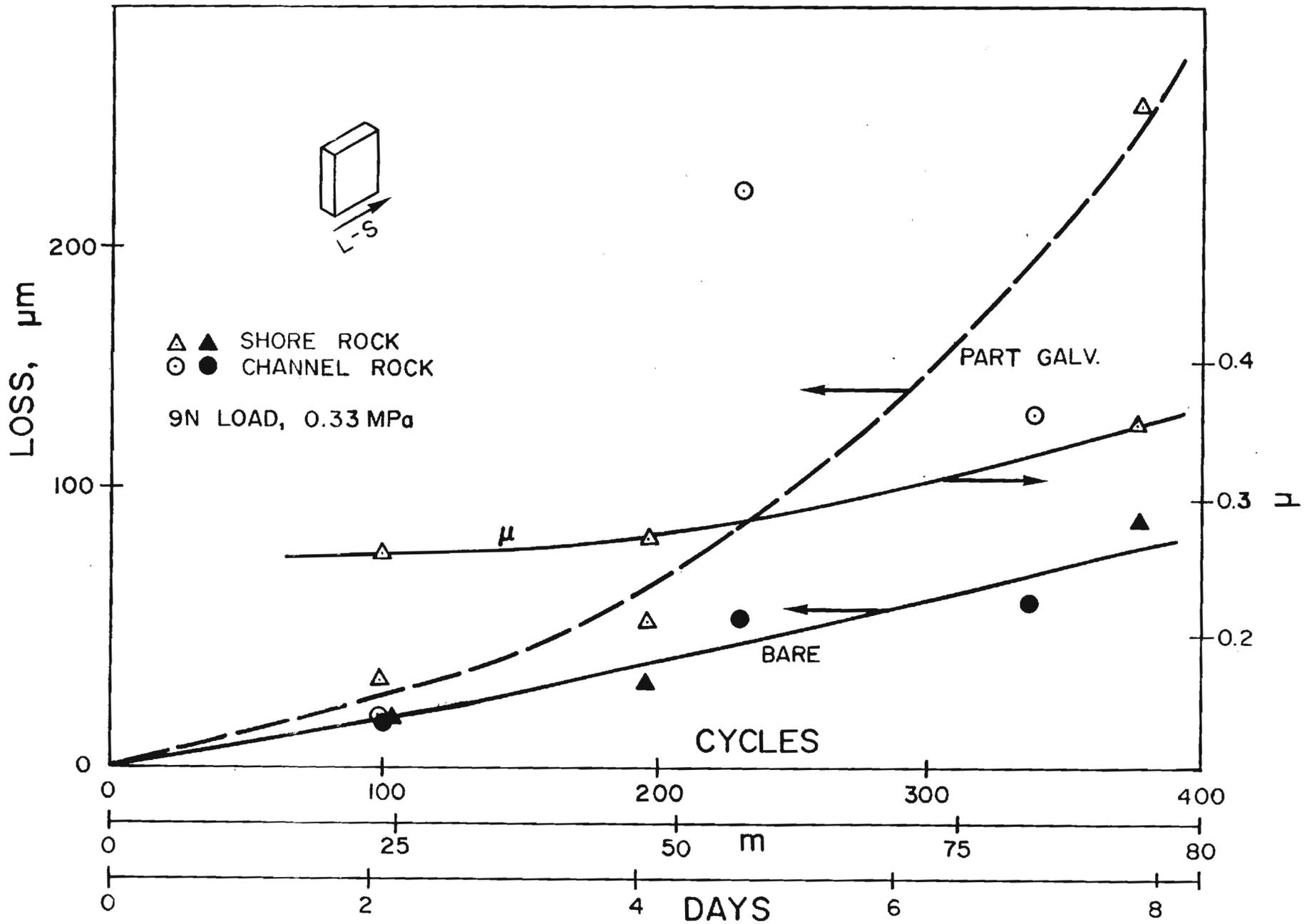
Fig. 23 Corrosion-erosion in stagnant seawater at room temperature.
