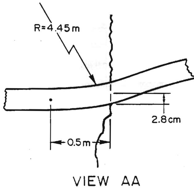
Fig. 5 Top view of catenary exposed to tidal current drag; excursion at mid-point, balance between tidal current drag and possible friction against rock; possible excursion at support point.
