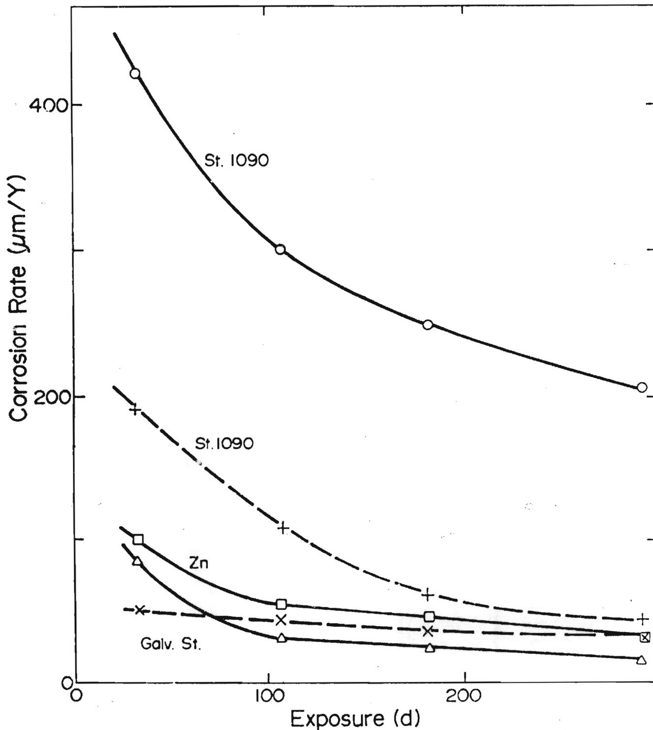
Fig. 4 Corrosion data for 0.9 % carbon steel, pure zinc, and galvanized steel exposed in slowly flowing Hawaiian surface seawater (25-28 °C, full lines) and cold (7-9 °C, dashed lines) deep ocean water pumped from 600 m depth /6/
