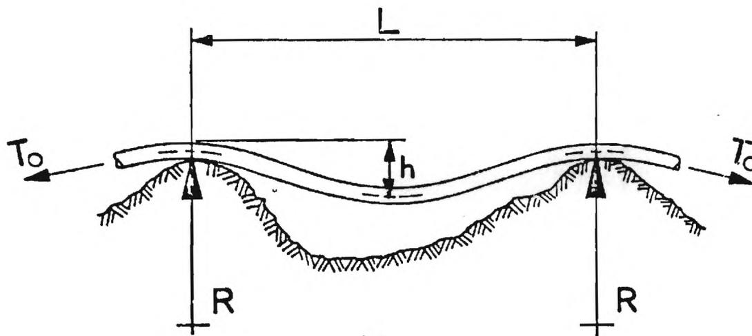
Fig. 1 Configuration of cable suspended on two outcrops of the same height
