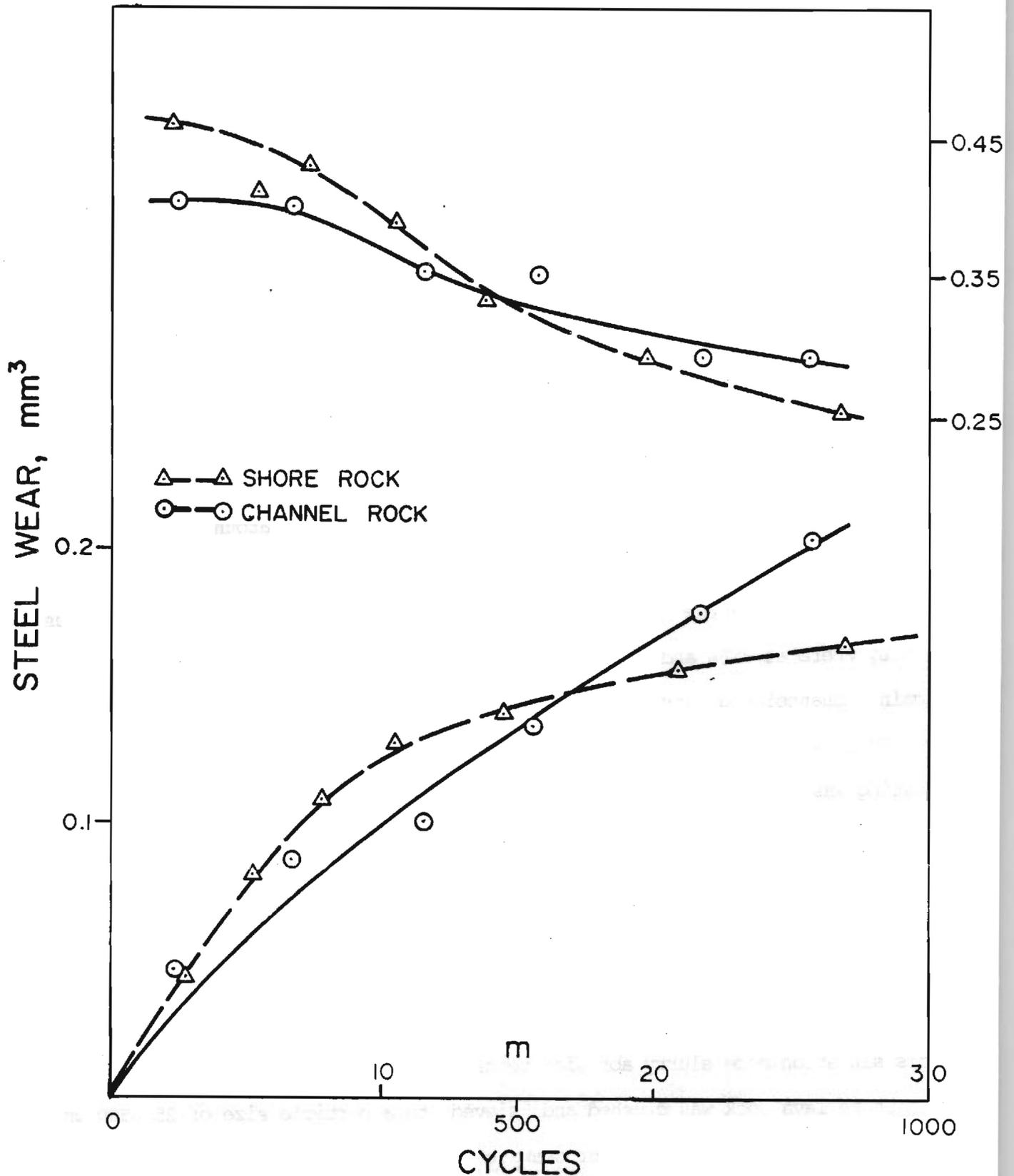
Fig. 20 Wear of bare armor wire abraded in the L-S direction against a 90° edge of rock under 46.4 N load.
