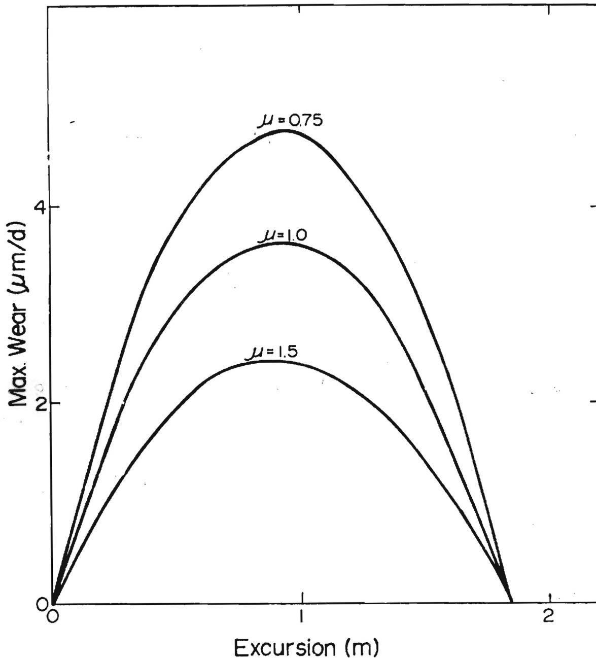
Fig. 5 Calculated maximum wear rates for assumed values of friction and excursion per cycle
