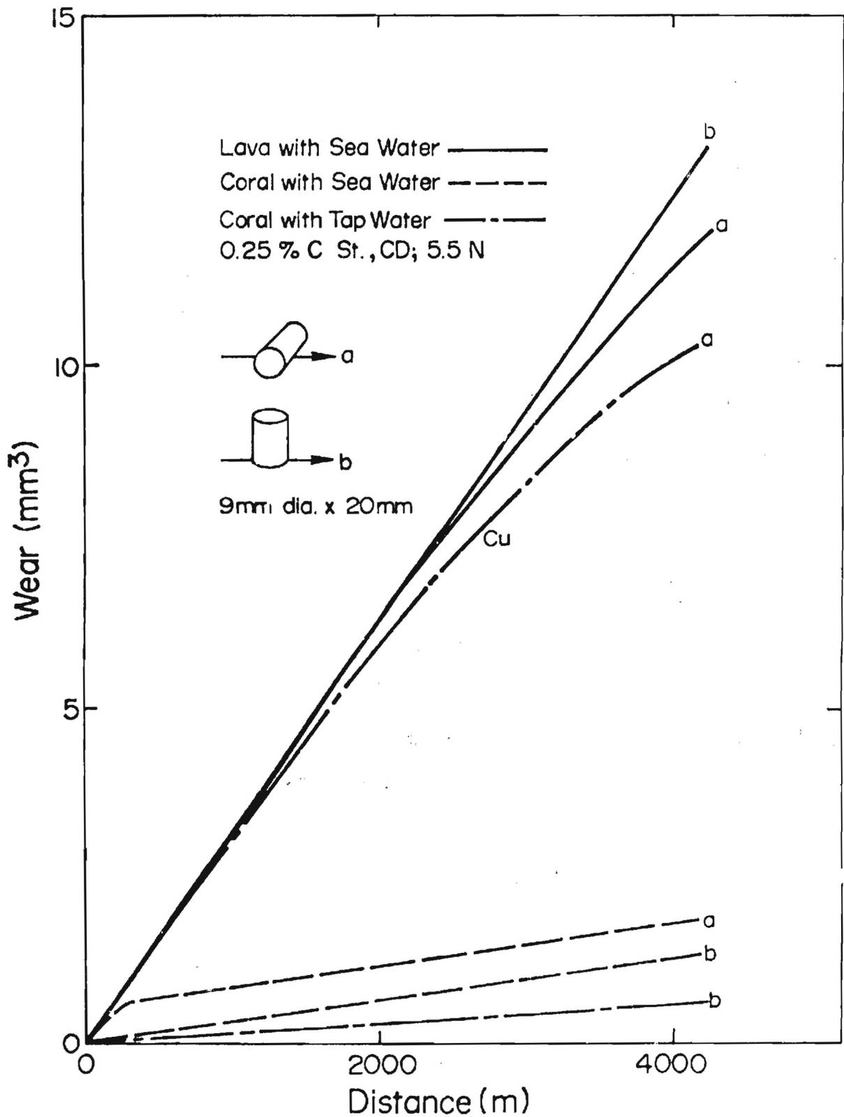
Fig. 3 Slurry abrasion data for copper and armor wire steel (cold drawn 0.25 %) in slurries of 250-400 crushed coral or lava with tap water or seawater. 4000 m sliding corresponds to 8.5 h of testing and to 7,160 to-and-fro strokes /5/
