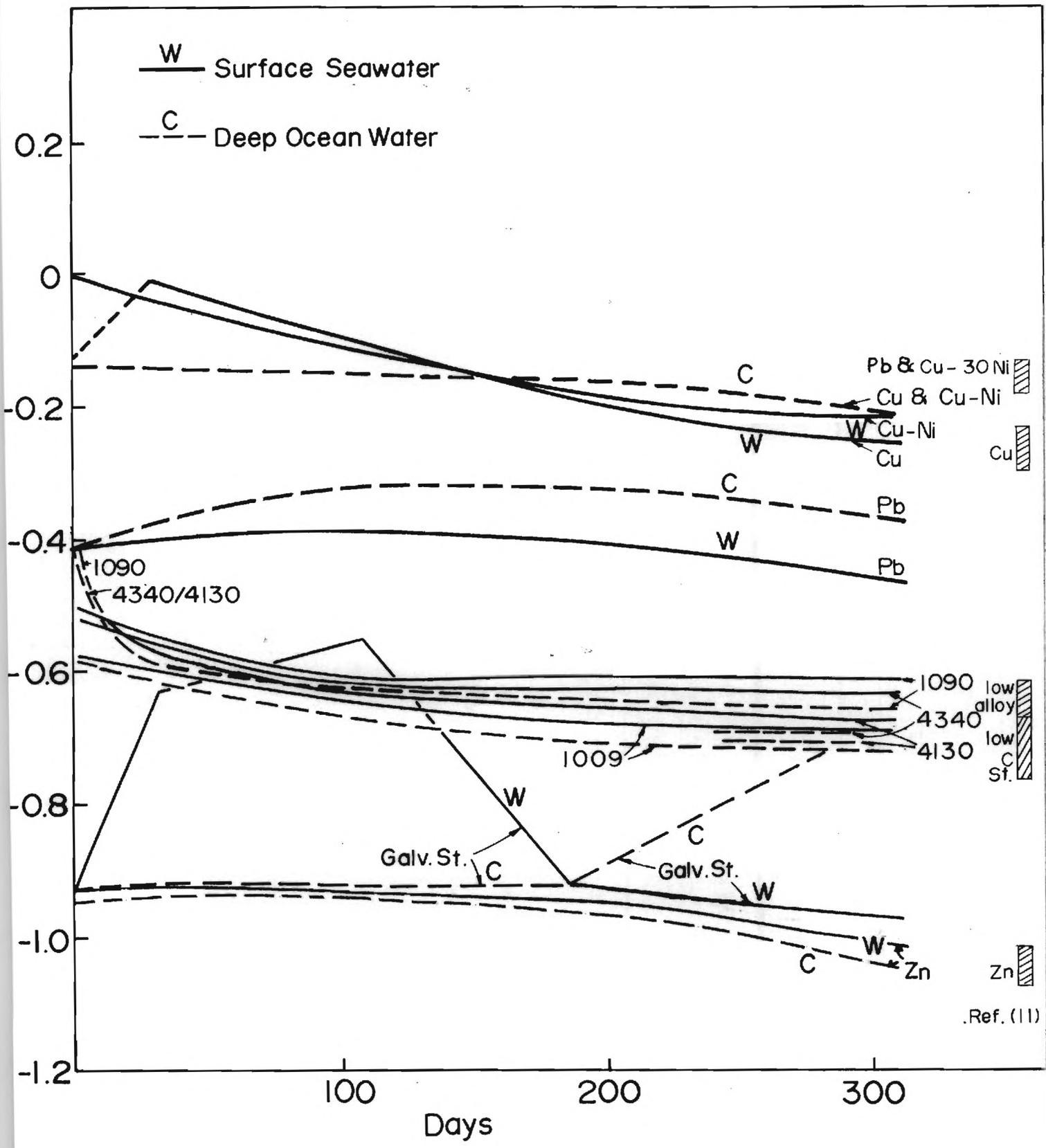
Fig. 1 Corrosion potentials, volts vs. Ag/AgCl for samples exposed in cold and warm water troughs at NELH (after Park). Comparison literature data for long-term exposures from the La Que Corrosion Center in North Carolina
