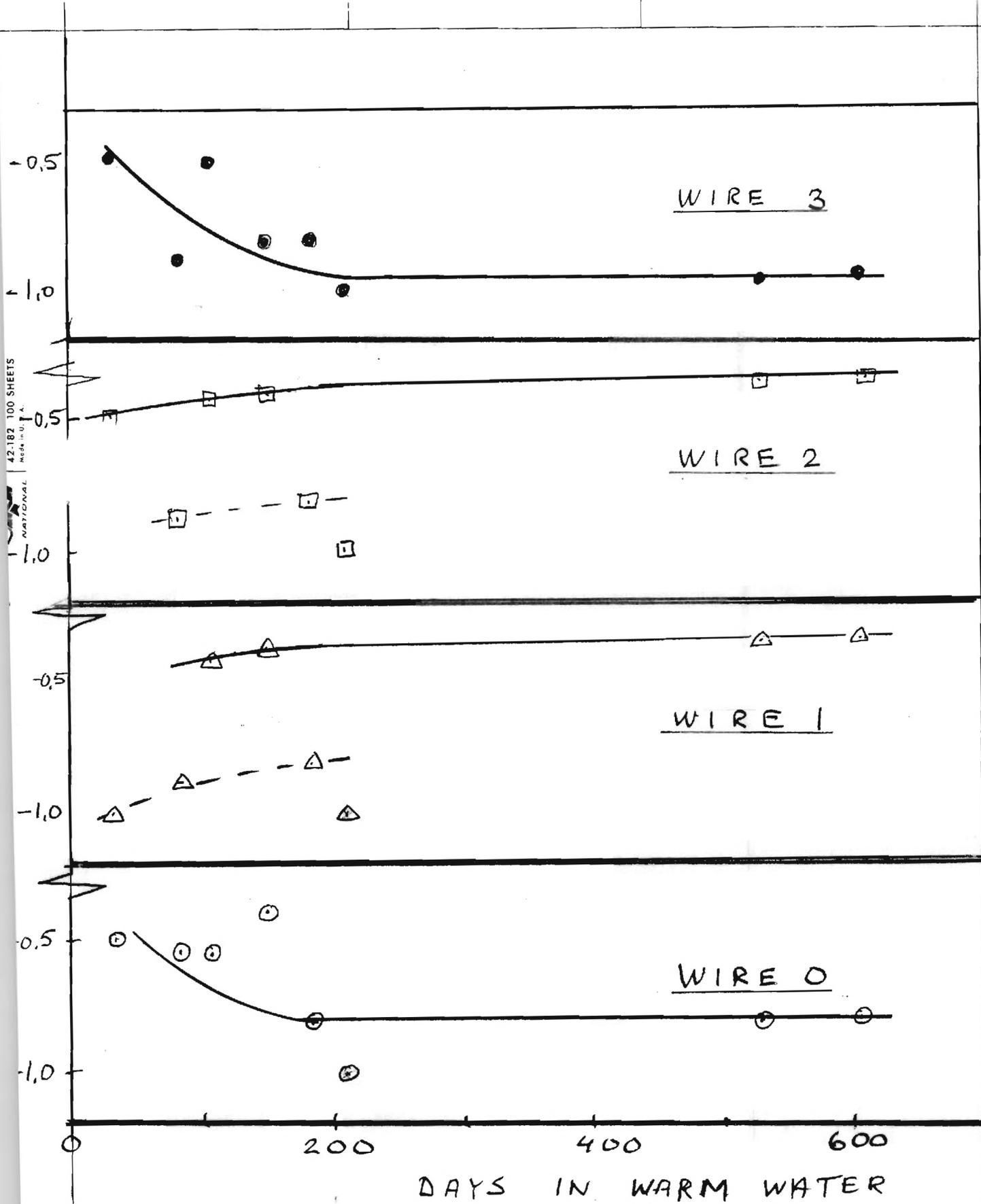
Fig. 2 Potentials,  $V$  vs.  $Ag/AgCl$ , of 4 different armor wires in cable specimen. Wires are cold drawn, galvanized AISI 1025 steel.
