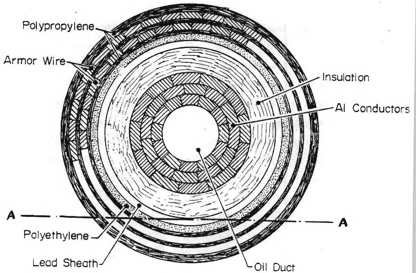
Fig. 2 Cross section of the final cable design. Only the major components are indicated.
