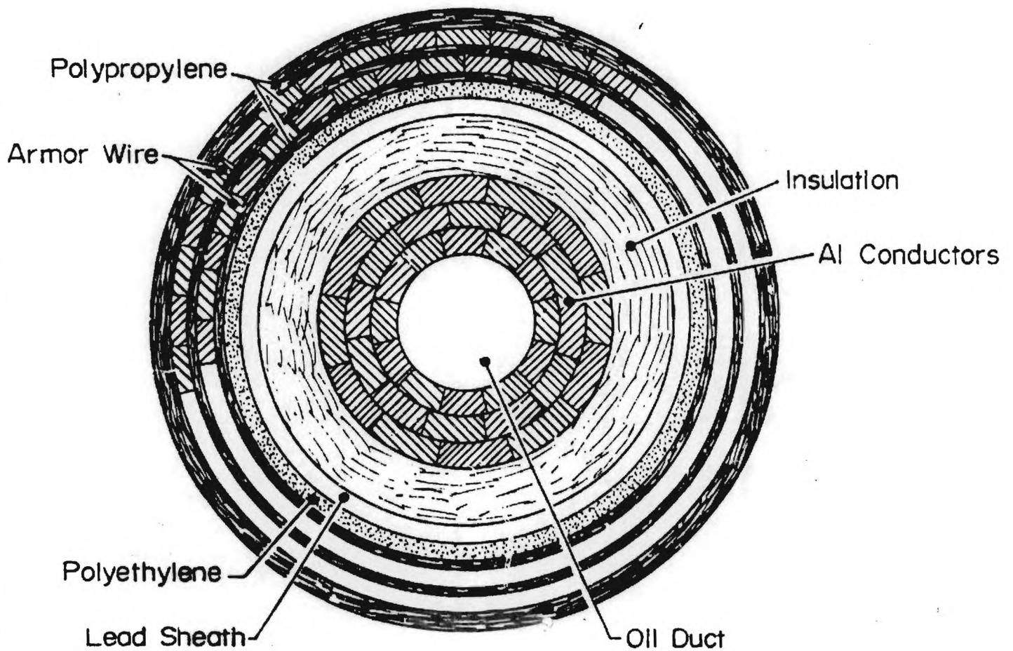
Fig. 2 Cross section of the final cable design. Cable is 300 kV d.c., self-contained oil filled. Weight in air: 37 kg/m. Weight in water 27 kg/m. Only the major components are indicated
