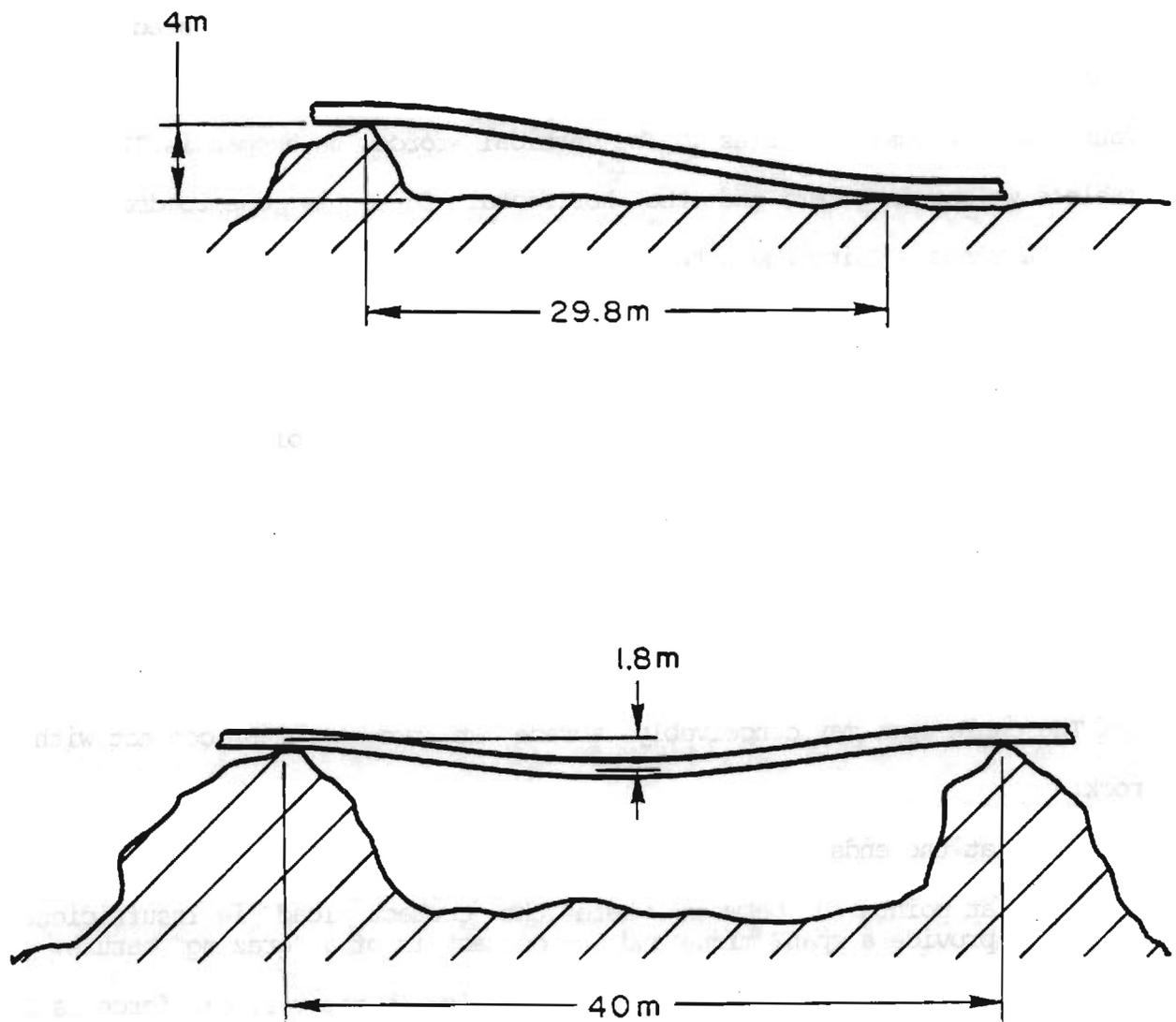
Fig. 4 Sketch of upper-limit conditions for which abrasion becomes a potential failure mechanism.
