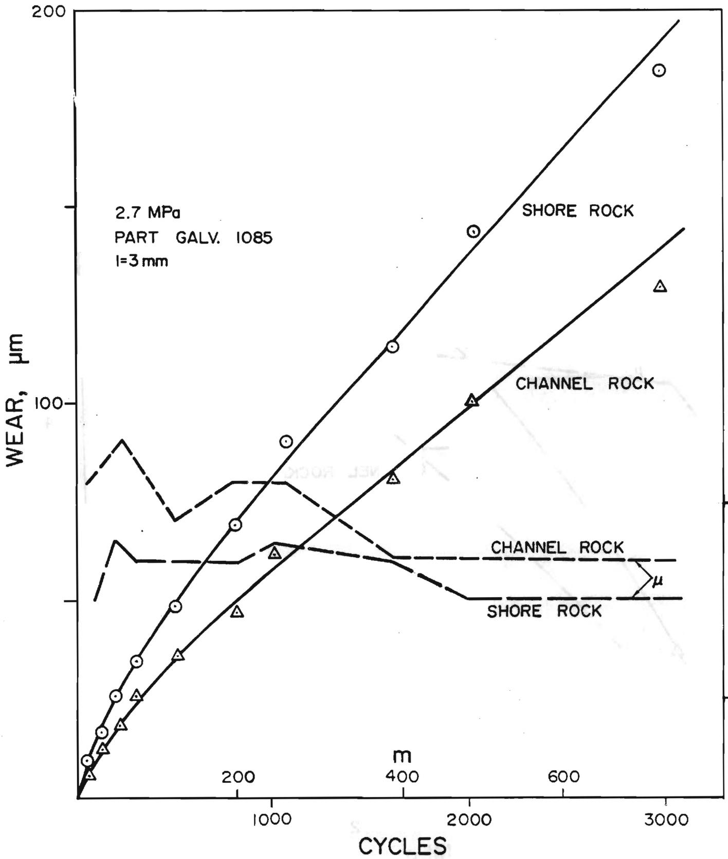
Fig. 19 Wear and coefficient of friction vs. sliding distance.
