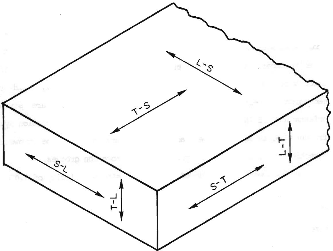
Fig. 11 Notations used to indicate sliding direction.
