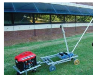
Mobile power supply designed for boom crane experiments in Dr. Bill Singhose's lab.
