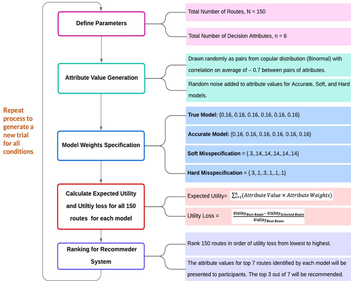
Figure 14. Steps to generate a set of 6 attribute values for the top 7 routes and top 3 recommended routes by an MDSS
