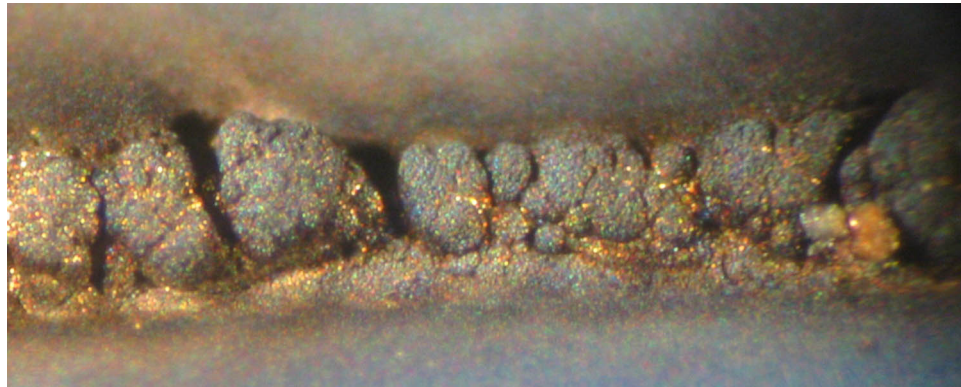
Figure 10.8: Optical image showing rough surface of 4-layer composite
