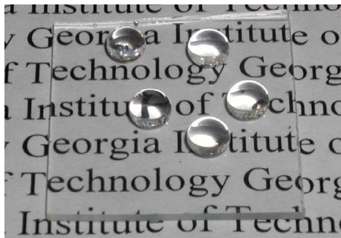
Figure 104. Optical demonstration of a transparent superhydrophobic silica film with dilution ratio ethanol: sol of 5:1 spin-cast at 3000 rpm.
