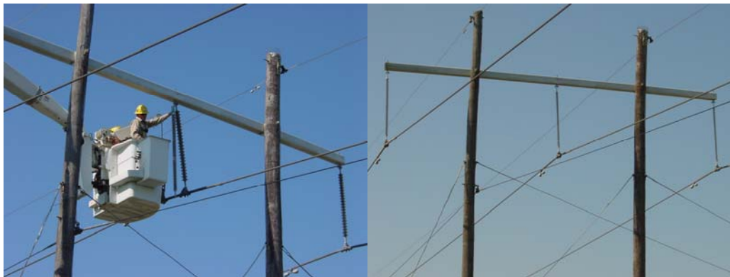
Figure 160. Field test of superhydrophobic coated insulators.
