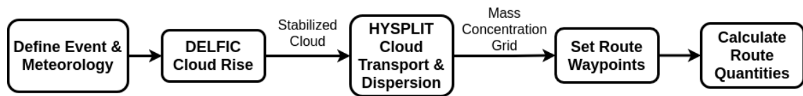
Figure 2.19: Typical workflow for a simulated problem in APTool. Radiological quantity computations are excluded for simplicity.
