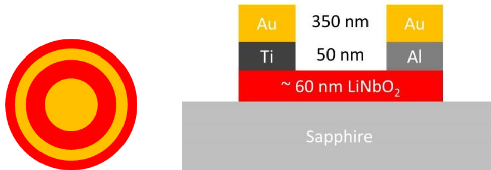
Figure 4-1. Non-volatile LiNbO 2 memristor device structure seen from above (left) and in cross-section (right). The outer ring and inner dot correspond to the Ti/Au and Al/Au contacts, respectively. Volatile memristors use Ti/Au for both contacts. The current convention is a positive bias on the outer ring electrode.
