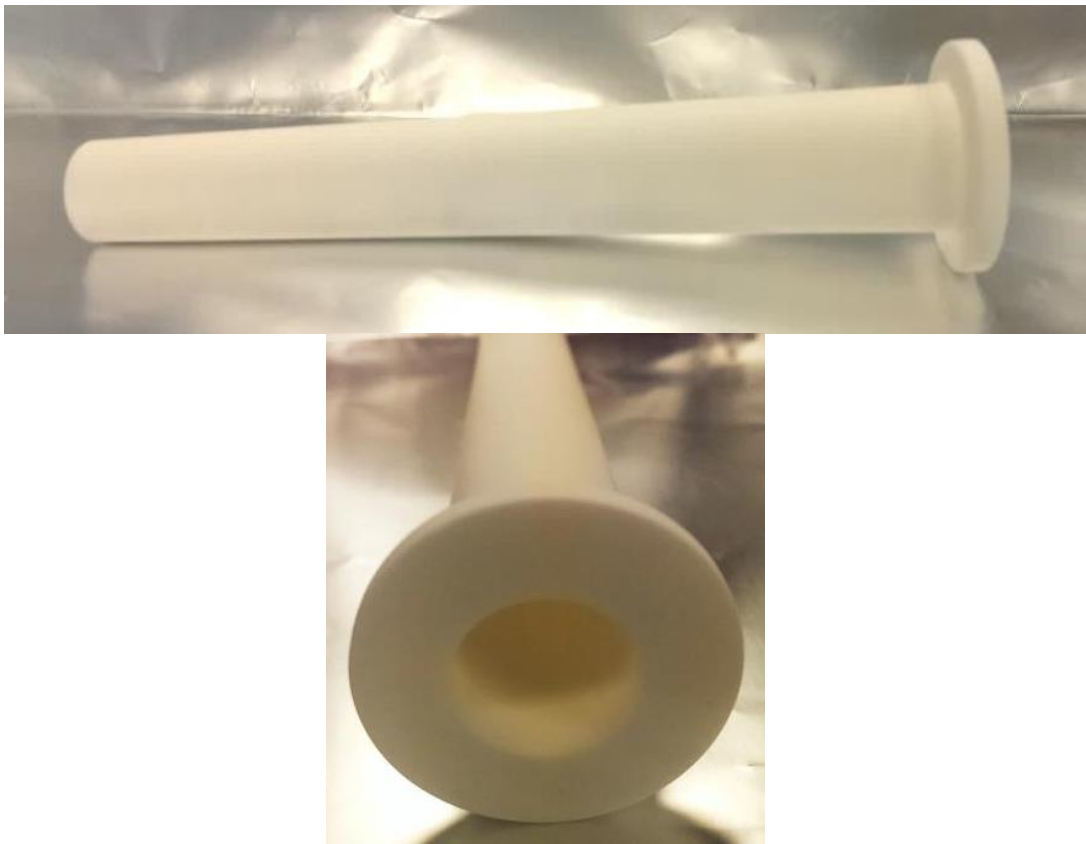
Figure 3-5. Custom beryllia crucible made to hold \text{LiClO}_4 in a Knudsen effusion cell. Previous work has indicated that \text{LiClO}_4 will corrode anything that can oxidize, and Li will intercalate into and swell PBN.
