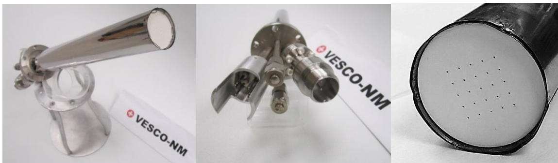
Figure 3-1. (left) Custom \text{NbCl}_5 cell with (center) tip filament, bulk water, tip and bulk thermocouple feedthroughs, and (right) a 5x5 hole pattern aperture plate.
