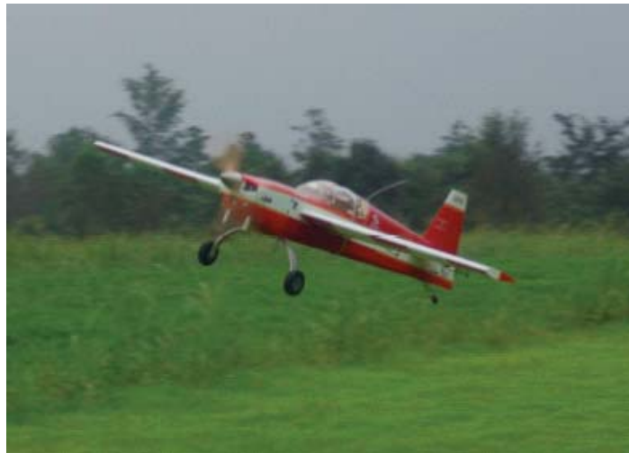
Figure 1. The GTEdge research UAV is a modified 33% scale Edge 540T. This vehicle was selected for its ability to carry moderate payloads and to perform aggressive aerobatic maneuvers. Vibration isolation and electromagnetic interference shielding protect the avionics mounted within the aircraft's canopy.
