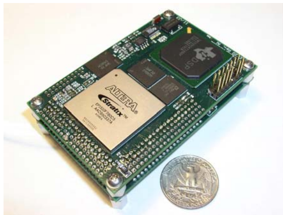
Figure 2. The FCS20 with EC20 Processor Board on top
