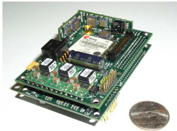
Figure 3. FCS20 with SB20 Sensor/Power Board on top
