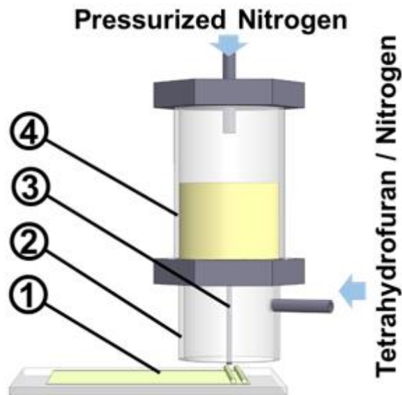
Figure 4. Schematic diagram of 3D-printing device: (1) Printing surface, (2) controlled atmosphere chamber, (3) printing nozzle, and (4) printing ink.
