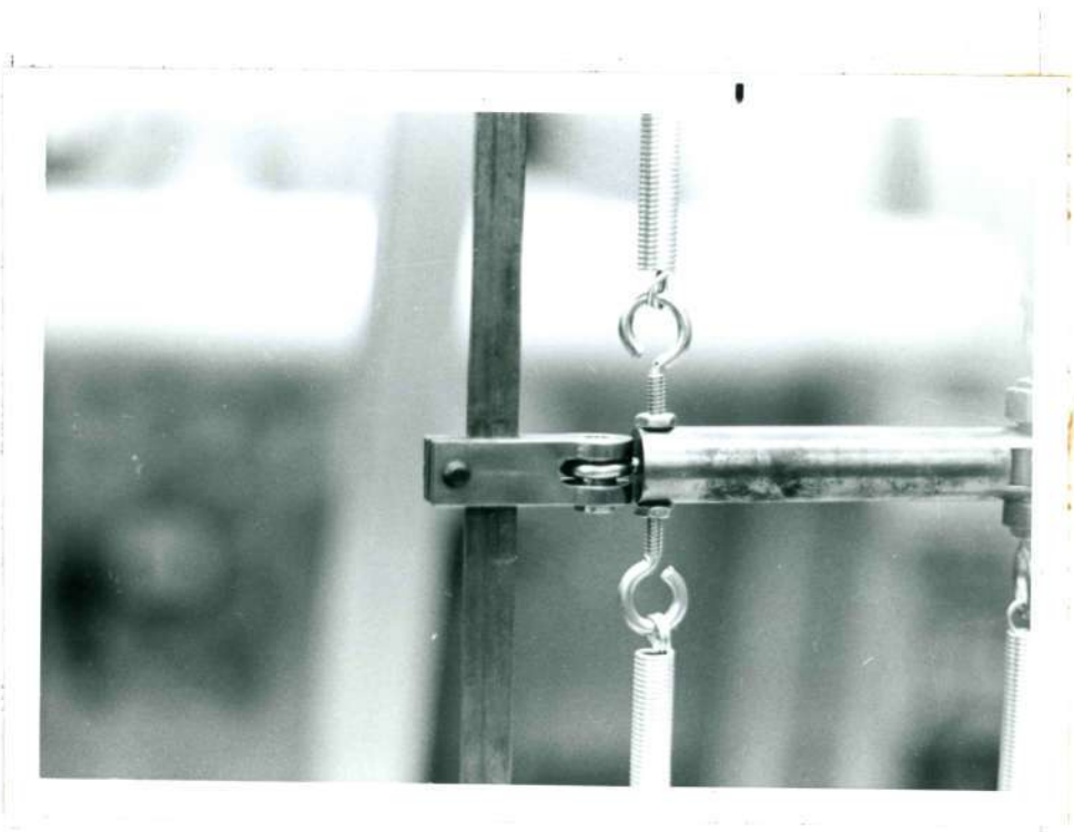
Figure 31. Coupling of Beam to Chain
