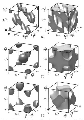
Fig. 1. (Color online) Four-beam interference resulting in (a) face-centered, (b) body-centered, and (c) simple cubic lattices. Isocontours are drawn to encompass volumes of material experiencing relatively high intensities. Solutions resulting in V>0 with intensity maxima (left) and in V<0 with intensity minima (right) located at lattice points. Optimized parameters for these solutions are summarized in Tables 1 and 2.
