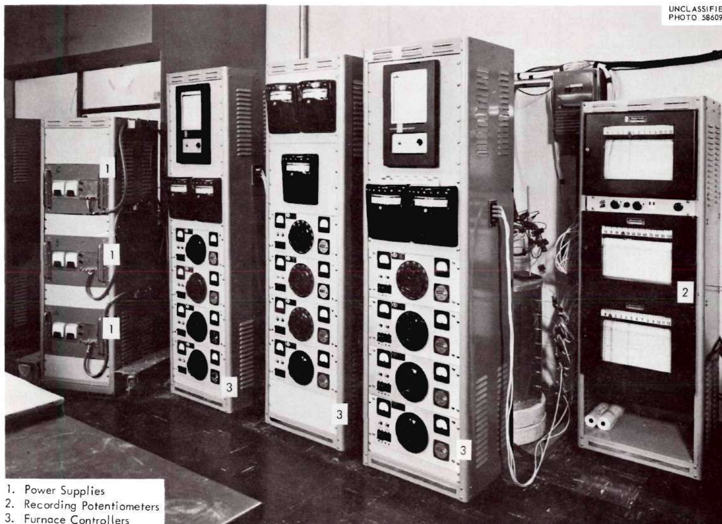
Fig. 48. Power Supplies, Furnace Controllers, and Recording Potentiometers.
