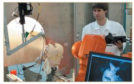
by designing and fabricating an improved knife end-effector and expanding the use of force control. The team also plans to perform a more extensive statistical study of bird features and further explore active wing manipulation.
