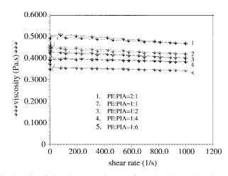
Fig. 2. Plot of viscosity versus shear rate for various PIA to PE ratios.
