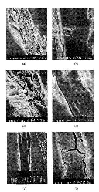
Fig. 6. SEM microstructure cross section analysis. (a), (c), (e) are the developed PIAE adhesives (PIA:PE = 1:1) exposed to curing temperature,  $350 \,^{\circ}C/1$  h, and  $400 \,^{\circ}C/1$  h, respectively. (b), (d), (f) are the commercial PIA adhesives exposed to curing temperature,  $350 \,^{\circ}C/1$  h, and  $400 \,^{\circ}C/1$  h, respectively.
