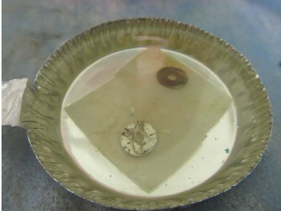
magnetic cores in final methy ethyl ketone (MEK) release
