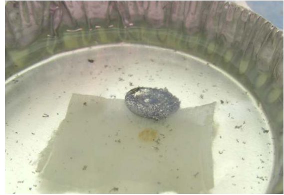
magnetic core disintegrating during final MEK release
