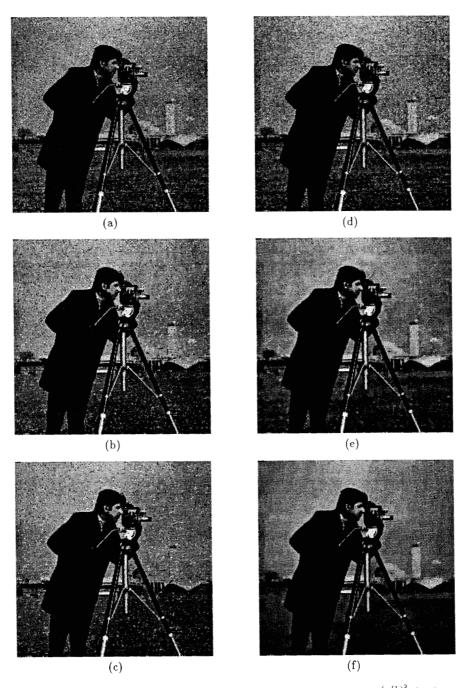
Figure 2: Scale spaces of Anisotropic Diffusion. Diffusion coefficient  $c(s) = \exp^{-(s/k)^2}$  for images in the left column,(a) t=5, (b) t=45, and (c) t=150. Diffusion coefficient  $c(s) = \frac{2}{3}s^{-4/3}$  for images in the right column, (d) t=10, (e) t=30, (f) t=50.
