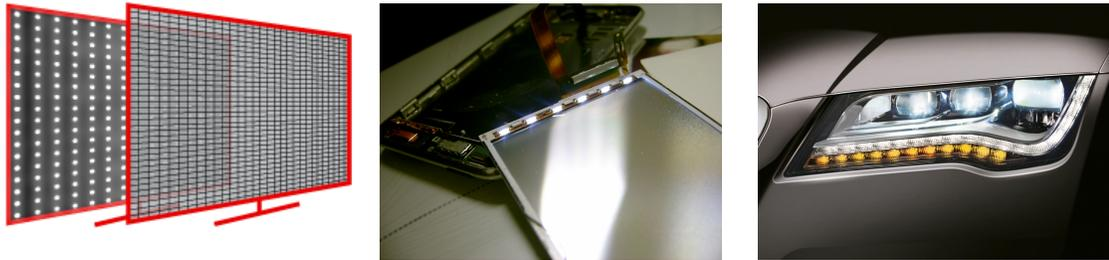
**Figure 1-1. LEDs in backlit TV, edge-lit mobile display, and automotive headlight [3].**
