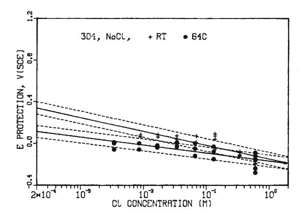
Fig. 11 - Protection potential data for Type 304 steel; standard conditions, room temperature and  $64^{\circ}C$ , regression lines.
