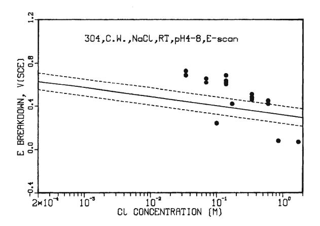
Fig. 3 - Breakdown potential data for Type 304 steel in aqueous chloride solutions; data for cold-worked materials superimposed on regression lines for standard conditions (annealed materials).
