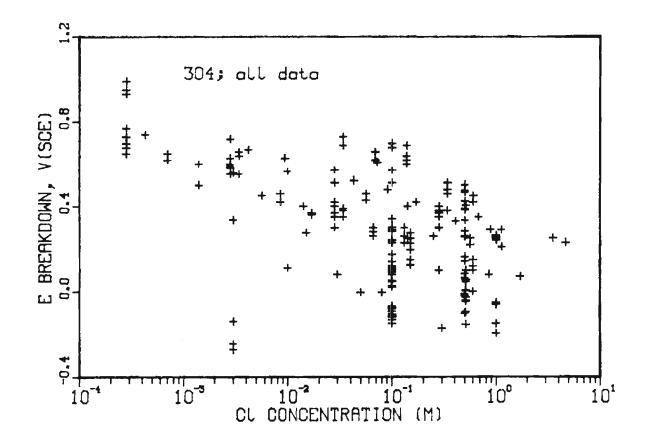
Fig. 1 - Breakdown potential data for Type 304 steel in aqueous chloride solutions; all data as a function of chloride ion concentration.
