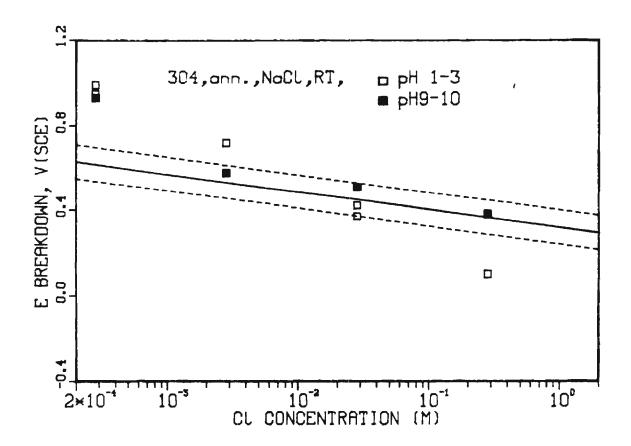
Fig. 5 - Breakdown potential data for Type 304 steel in aqueous chloride solutions; data for low and high pH solutions, superimposed on regression lines for standard conditions (pH 4 - 8).
