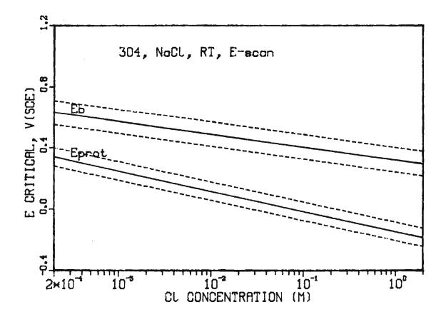
Fig. 12 - Regression lines for breakdown and protection potential data for Type 304 steel, standard conditions.
