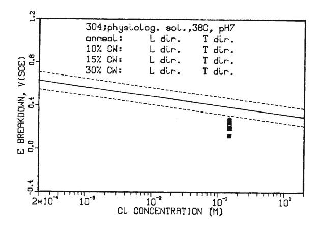
Fig. 6 - Breakdown potential data for Type 304 steel in aqueous chloride solutions; data for physiological solution, 38°C, and different amounts and directions of cold-work, superimposed on regression lines for standard conditions (aqueous NaCl, room temperature, annealed).
