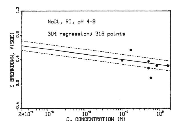
Fig. 8 - Breakdown potential data for Type 316 steel in aqueous chloride solutions; data for standard conditions, superimposed on regression lines for Type 304 steel data, standard conditions.
