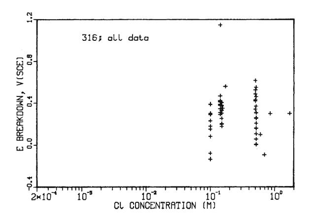
Fig. 7 - Breakdown potential data for Type 316 steel in aqueous chloride solutions; all data as a function of chloride ion concentration.
