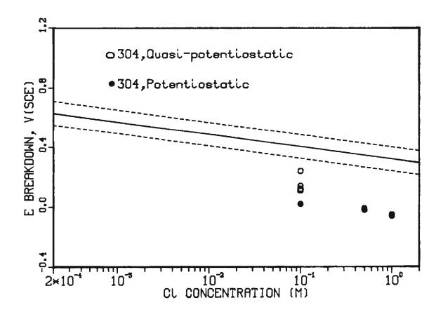
Fig. 4 - Breakdown potential data for Type 304 steel in aqueous chloride solutions; data obtained by potentiostatic and quasipotentiostatic techniques, superimposed on regression lines for standard conditions (potentiodynamic techniques).
