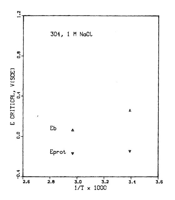
Fig. 13 - Breakdown and protection potential data for Type 304 steel, standard conditions, normalized to 1 M concentration, as a function of absolute temperature.
