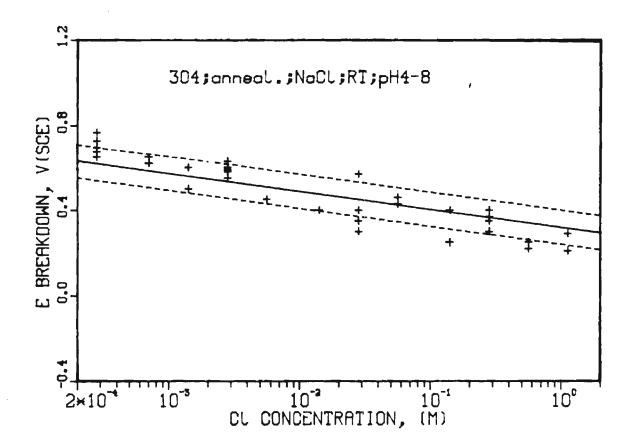
Fig. 2 - Breakdown potential data for Type 304 steel in aqueous chloride solutions; data for standard conditions as a function of chloride ion concentration; regression lines.
