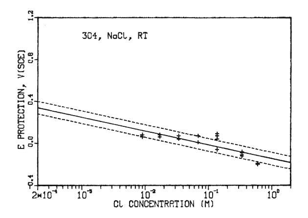
Fig. 10 - Protection potential data for Type 304 steel; data for standard conditions as a function of chloride ion concentration, regression lines.
