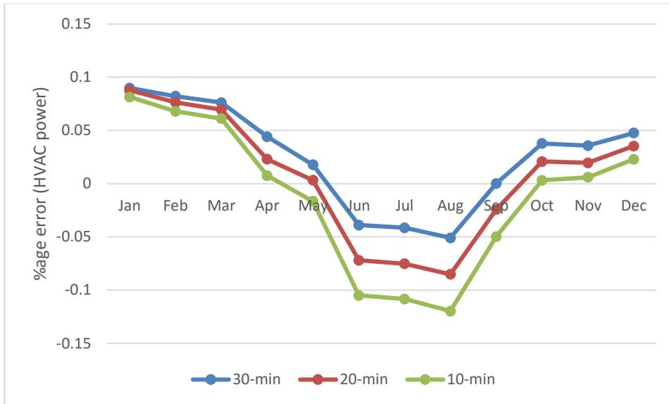
Figure 3.25: Percentage error for DX cooling HVAC power consumption values by decreasing timestep, Chicago, IL
