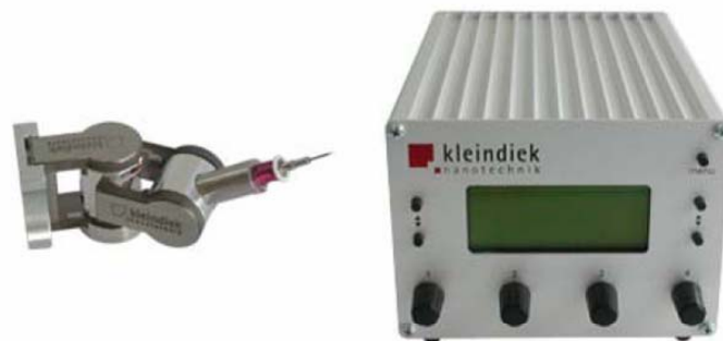
Figure 34: Photo of the micro-manipulator and the control electronic system from Kleindiek.
