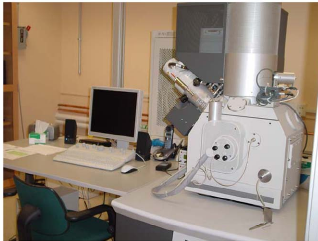
Figure 33: Photo of Nova dual beam focus ion beam machine.
