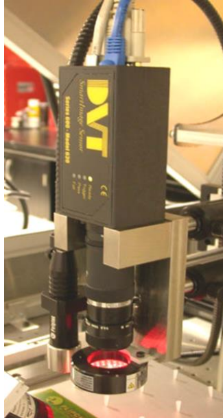
Figure 41 – DVT series 600 smart sensor camera for locating fiducial marks
