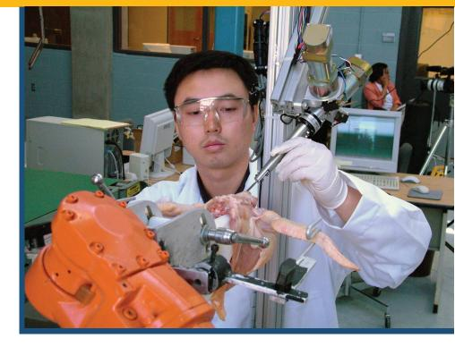
The 2-axis manipulator uses a force-torque sensor to determine forces at the knife, and the controller adjusts the path of
