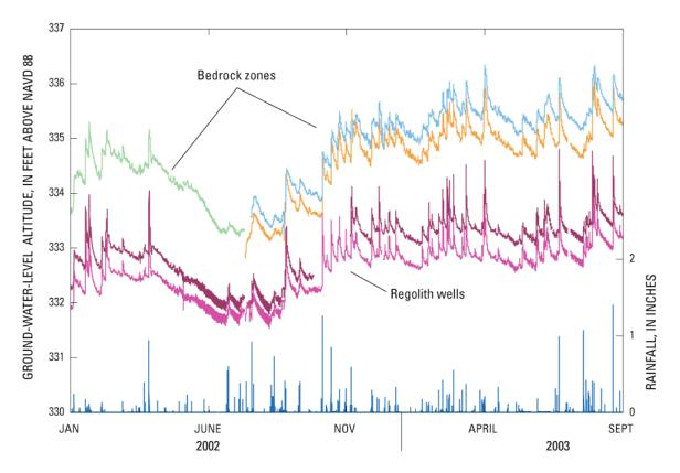
Figure 4. Continuous ground-water levels recorded in a discharge area at the Lake Wheeler Road research station, North Carolina (NAVD 88, North American Vertical Datum of 1988).
