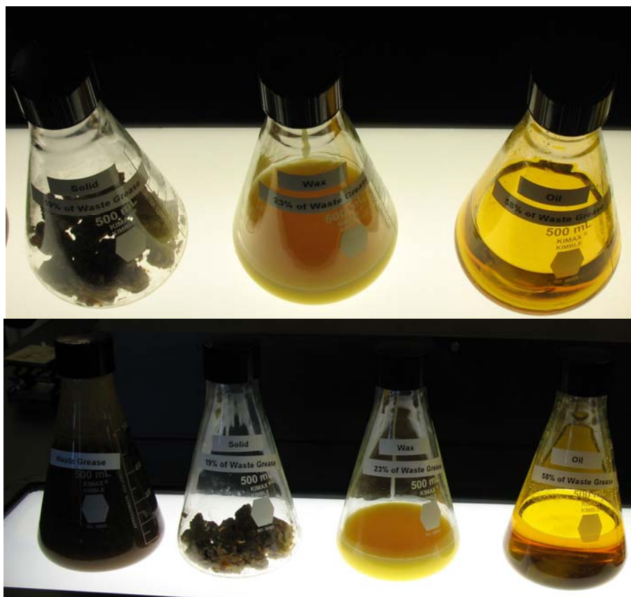
Figure 5.4 – (top) Photograph of three separated phases of polished brown grease: solids (left), wax (center), oil (right); (bottom) the three phases of PBG on the right with the unpolished brown grease on the far left.
