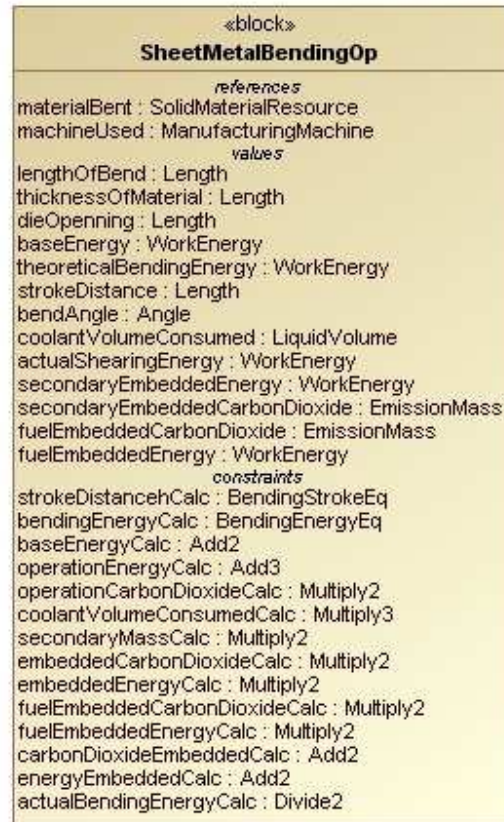
Figure A 13: Sheet metal bending operation block
