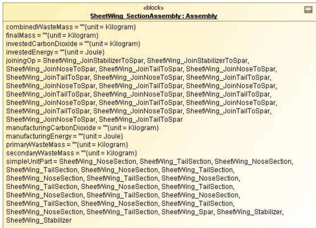
Figure A 36: Sheet metal wing assembly
