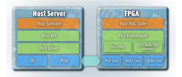
Figure 5.1: The vendor implemented Pico framework software stack gives easy to use APIs to tweak hardware design parameters on the FPGA logic. The stream framework may be used to interact directly with the HMC. Adopted from [15]
