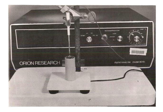
Fig. 8. Setup for pH Analysis of Microliter Samples Using an Inverted pH Electrode.
