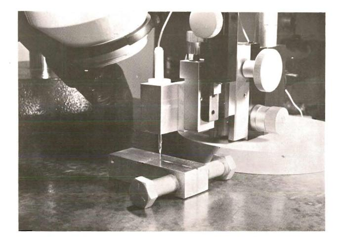
Fig. 4. Experimental Setup for Application of Microprobes in Cracks (Detail).
