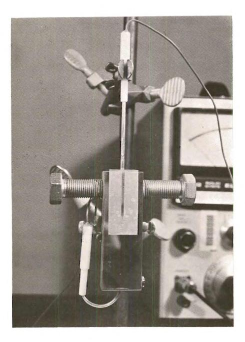
Fig. 13. Setup for Measurement of the Potential at the Crack Tip Using an Implanted Electrode.
