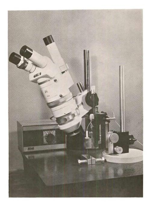
Fig. 3. Experimental Setup for Application of Microprobes in Cracks.
