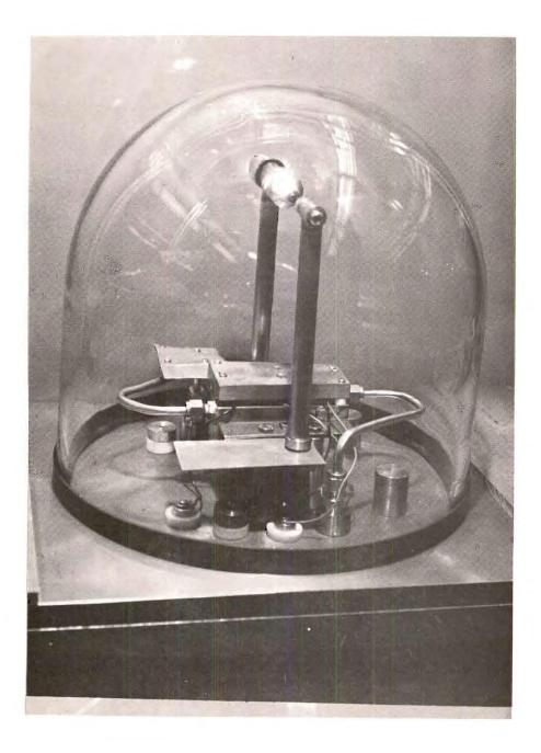
Fig. 5. Vacuum Chamber Used for Freeze-Drying of the Electrolyte.
