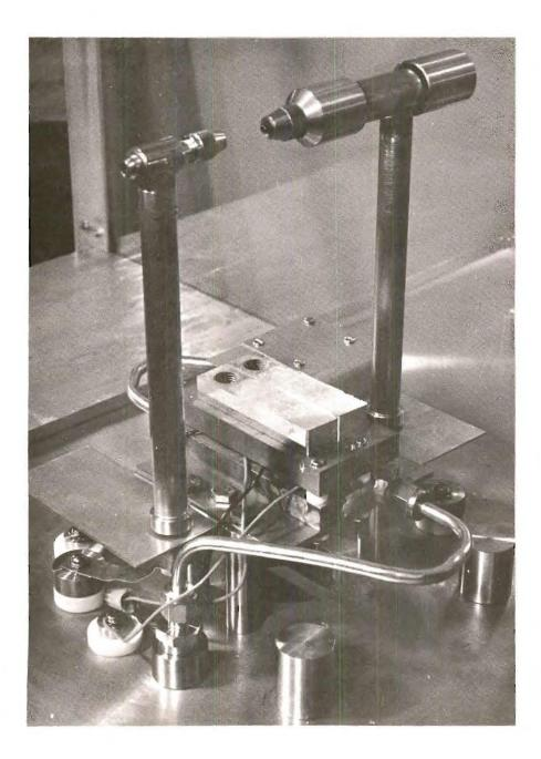
Fig. 6. Thermoelectrically Cooled Stage and Carbon Evaporator Used in the Freeze-Dry Technique.
