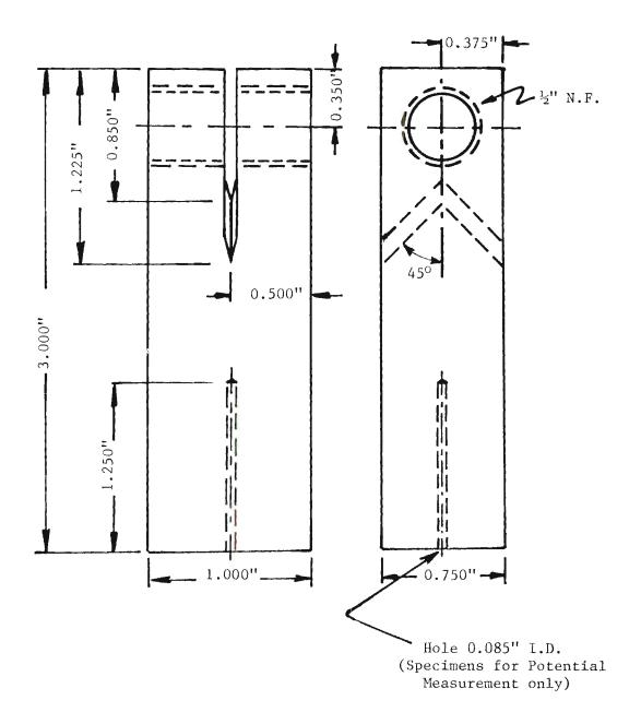
Fig. 1. SCC Specimen for the Determination of Electrochemical Conditions within cracks.
