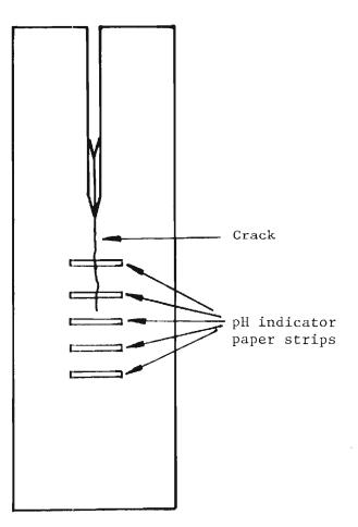
Fig. 7. Schematic Illustration of the Location of Indicator Strips for Determination of Crack Tip Acidity.
