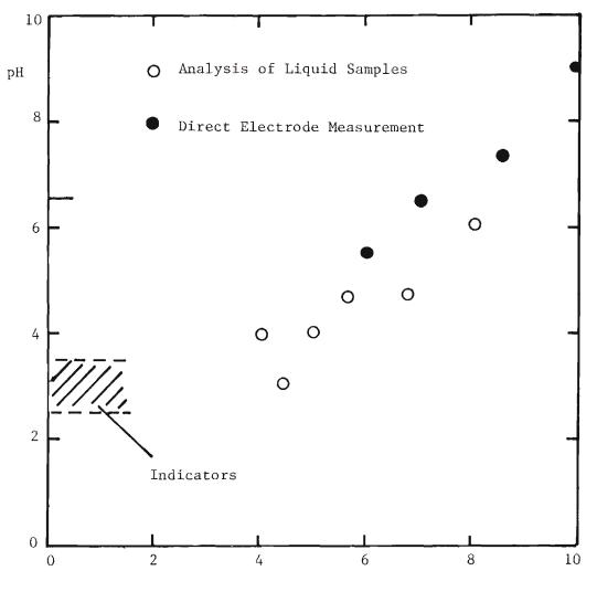
Distance from Crack Front (mm)
