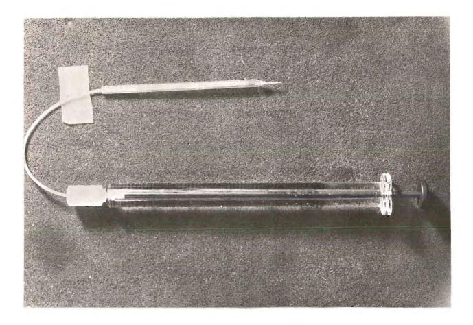
Fig. 2. Microcapillary Probe for Collection of Liquid Samples from Cracks.
