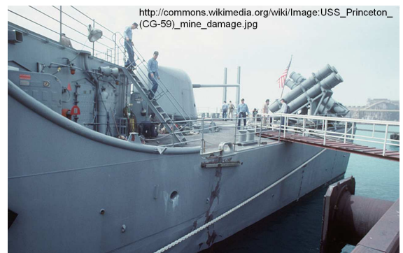
(b) USS Princeton (CG-59) with Mine Damage (1991)
