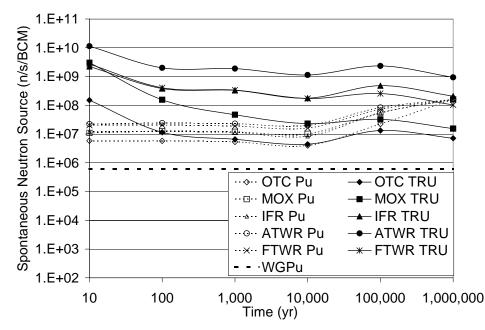
Figure 12 - Spontaneous Neutron Source From One Bare Critical Mass (dashed lines - plutonium only; solid lines - all transuranics)
