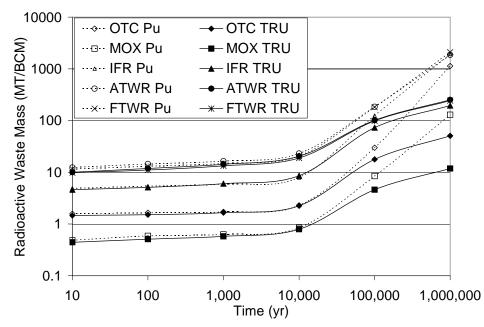
Figure 13 - Mass of Radioactive Waste Containing One Bare Critical Mass (dashed lines - plutonium only; solid lines - all transuranics)
