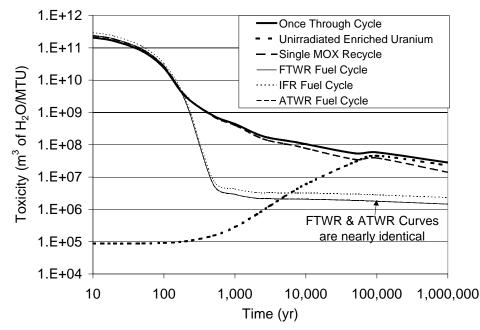
Figure 3 - Toxicity of Waste Sent to Repository per Unit Mass of LWR SNF
