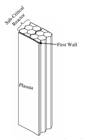
Figure 16 - Transmutation Reactor Configuration Outboard of Plasma Chamber
