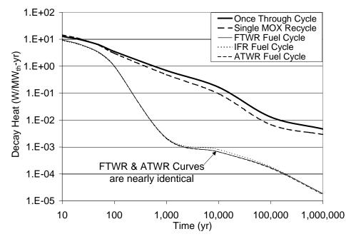
Figure 8 - Rate of Production of Decay Heat
