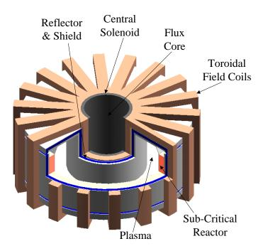
Figure 15 - Fusion Transmutation of Waste Reactor Schematic
