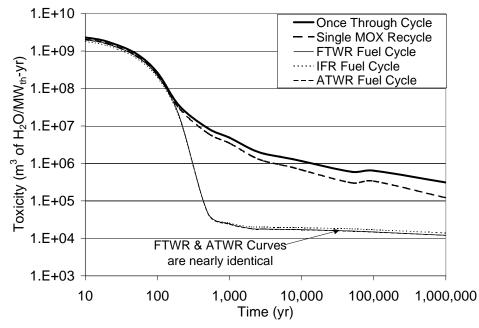
Figure 4 - Toxicity of Waste Sent to Repository per Unit Thermal Energy
