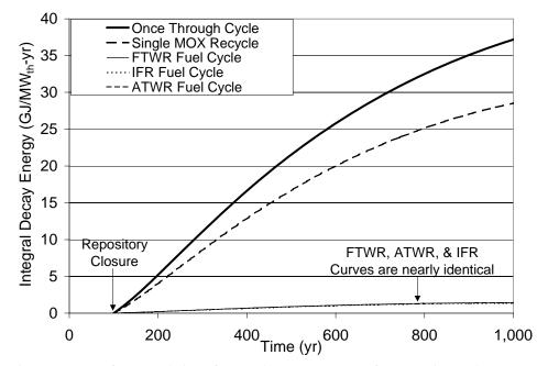
Figure 9 - Rate of Accumulation of Integral Decay Energy (After Repository Closure at 100 years)
