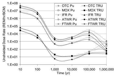
Figure 14 - Radiation Barrier of Waste Containing One Bare Critical Mass (dashed lines - plutonium only; solid lines - all transuranics)
