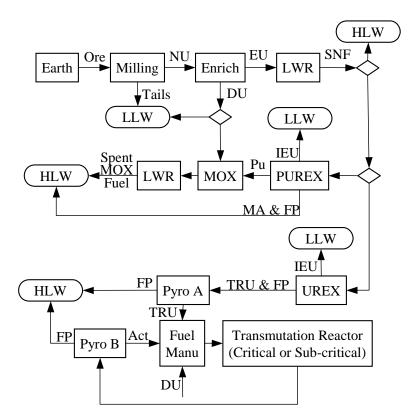
Figure 1 - Fuel Cycle Material Flow Diagram
