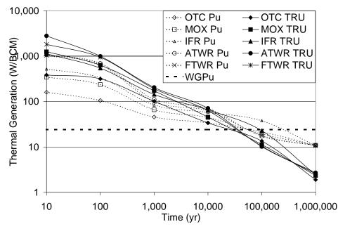
Figure 11 - Decay Heat From One Bare Critical Mass (dashed lines - plutonium only; solid lines - all transuranics)
