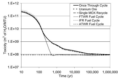
Figure 5 - Toxicity Of All Waste Streams From 1 Ton Of Enriched Uranium
