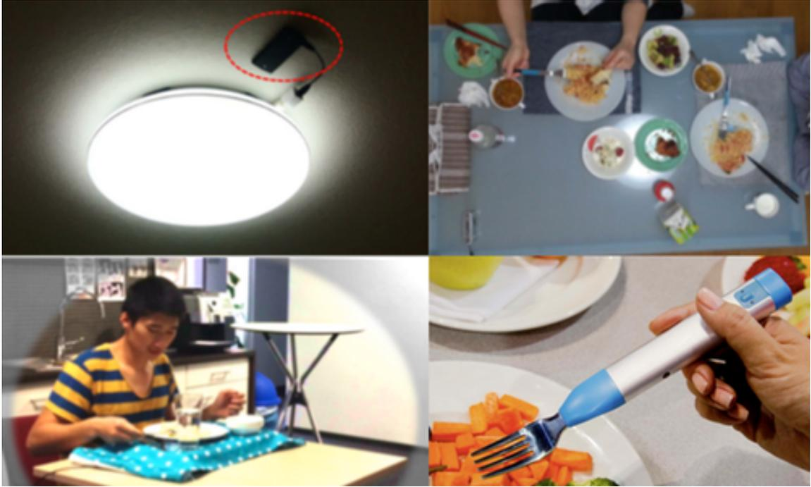
Figure 3: The top row images show the ceiling light camera by Maekawa and a typical photo taken with the camera [83]. The bottom-left image is showing the smart table surface by Zhou et al. [147]. The HAPIfork is shown in the bottom-right picture.
