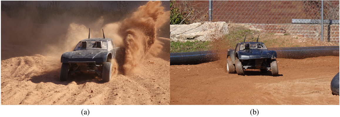
Figure 4.30: Examples of track surface variability during testing. (a) A dry and dusty track where traction is low. (b) A wet but not muddy track that offers a high traction environment surface.
