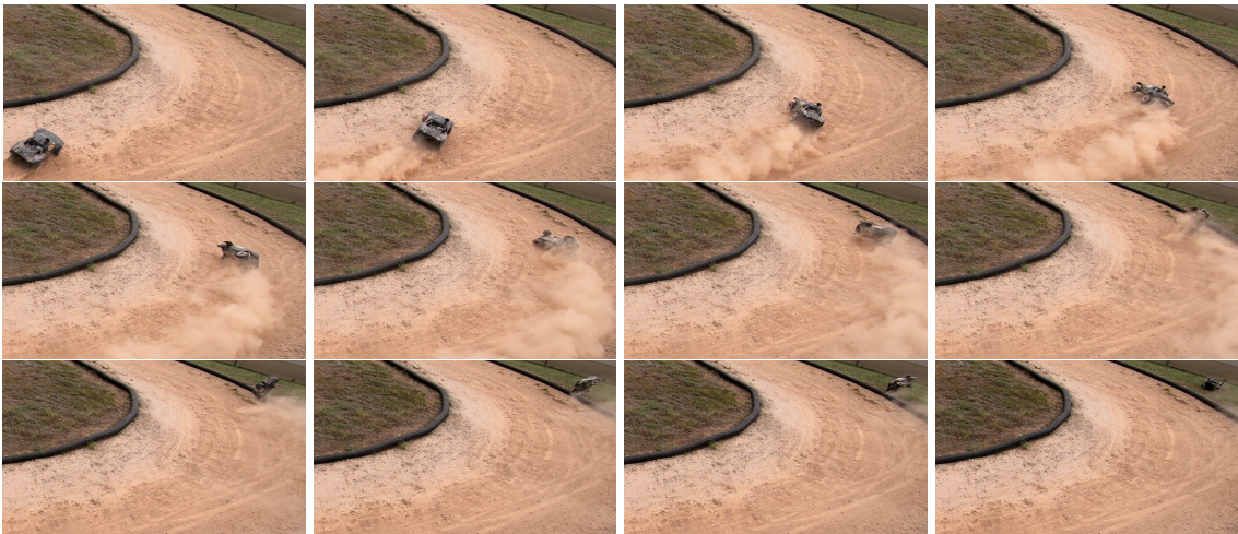
Figure 4.23: Sequence of images captured from offboard video of a multiple rollover crash during cost function optimization at GT-ARF large track. The crash was a result of excessive speed and side slip going through a turn.
