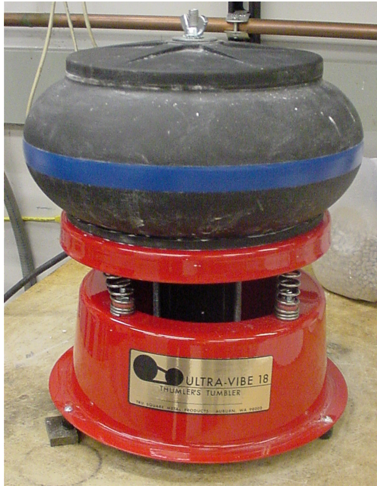
Figure 5.2: Ultra-Vibe 18 bowl-type vibratory tumbler
