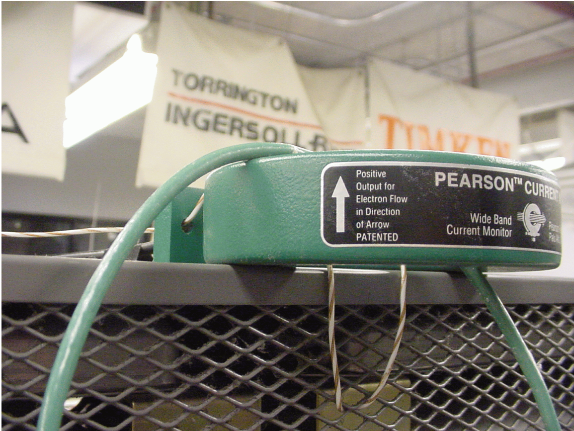
Figure A.7: All wires must be passed through the current sensor in the same direction
