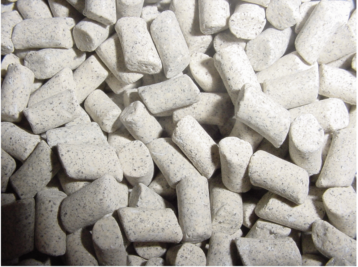
Figure 5.4: Photograph of coarse 22° ended cylinder preformed ceramic abrasive vibratory tumbling media
